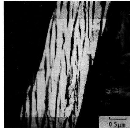
Fig. 7: Transmission electron micrograph of a mixture of bainitic ferrite and stable austenite.
