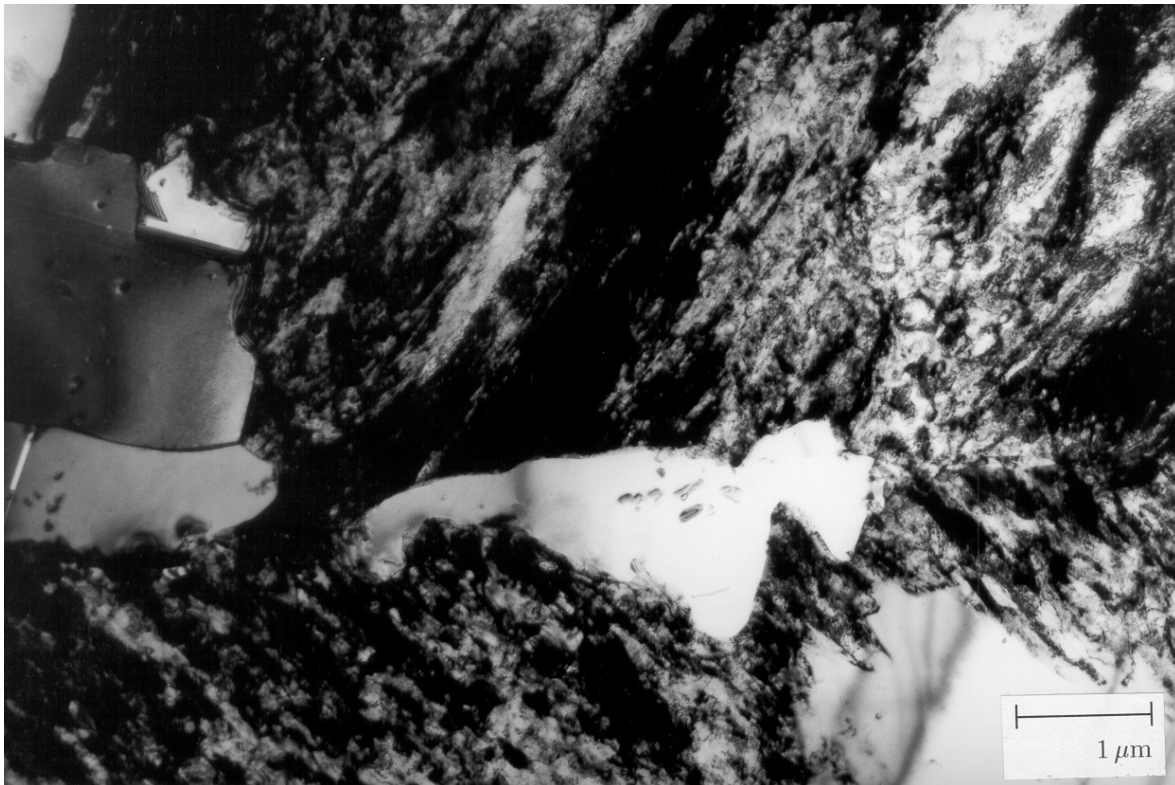
Fig. 4.6 A TEM micrograph from a type 302 stainless steel annealed for 1 hour at 685 °C illustrating nucleation occurring on the grain boundaries of the deformed structure
