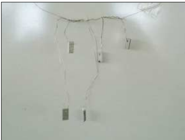
Fig. 1 – 5 samples prepared for suspension in the vertical furnace
