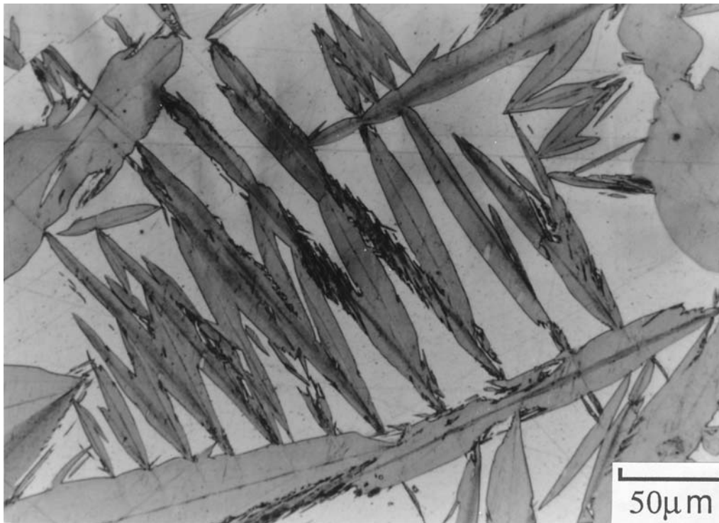
Fig. 2.21 A burst of autocatalytic martensitic transformation in a Fe-30Ni-0.31C wt% alloy. Such bursts are not observed during bainitic transformation.
