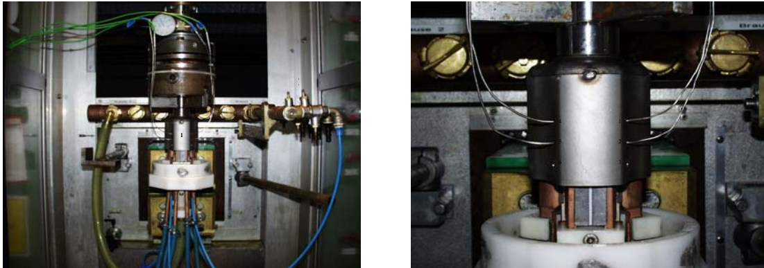
Figure 6.5: Experimental arrangement for temperature measurement during induction hardening
