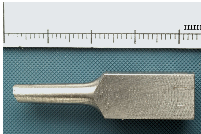
Figure 5.13: No necking is observed implying the elongation is mostly uniform.
