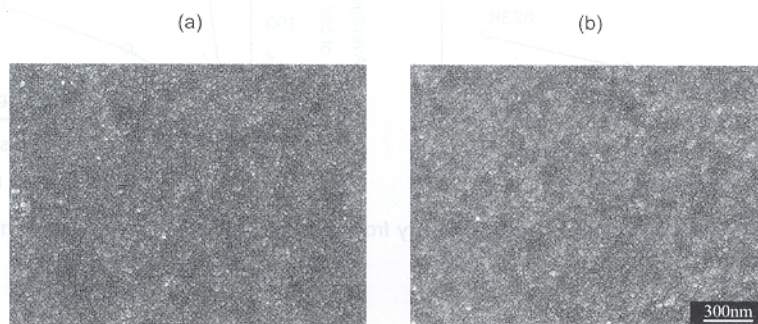
Fig.5. SEM images in non-cellular matrix of (a) 3.8Al and (b) 4.2Al alloy after ageing at 873 K.
