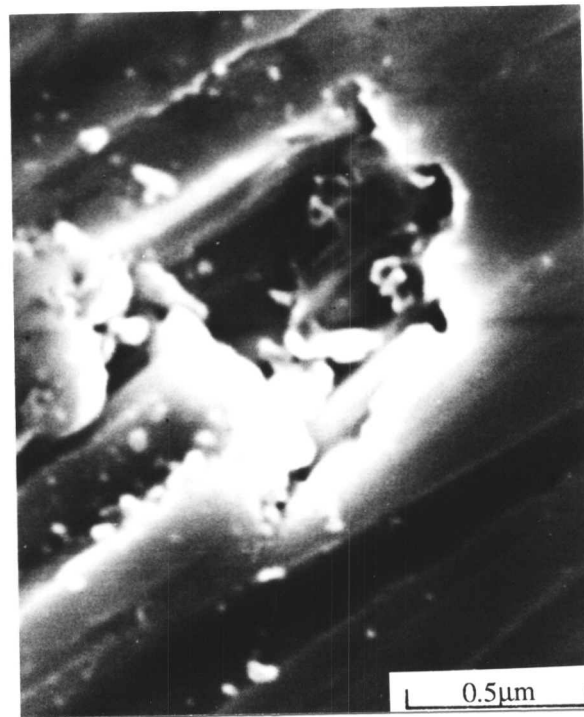
Fig. 7.9: Scanning electron micrographs of the worn surfaces of alloy 78 after the pin-on-disc abrasion test using; a) SiC (220 mesh) abrasives at 1kg load showing that carbides are worn to the same level as the matrix; b) \text{Al}_2\text{O}_3 (400 mesh) at 450g, showing pit formation along the carbide-matrix interface.
