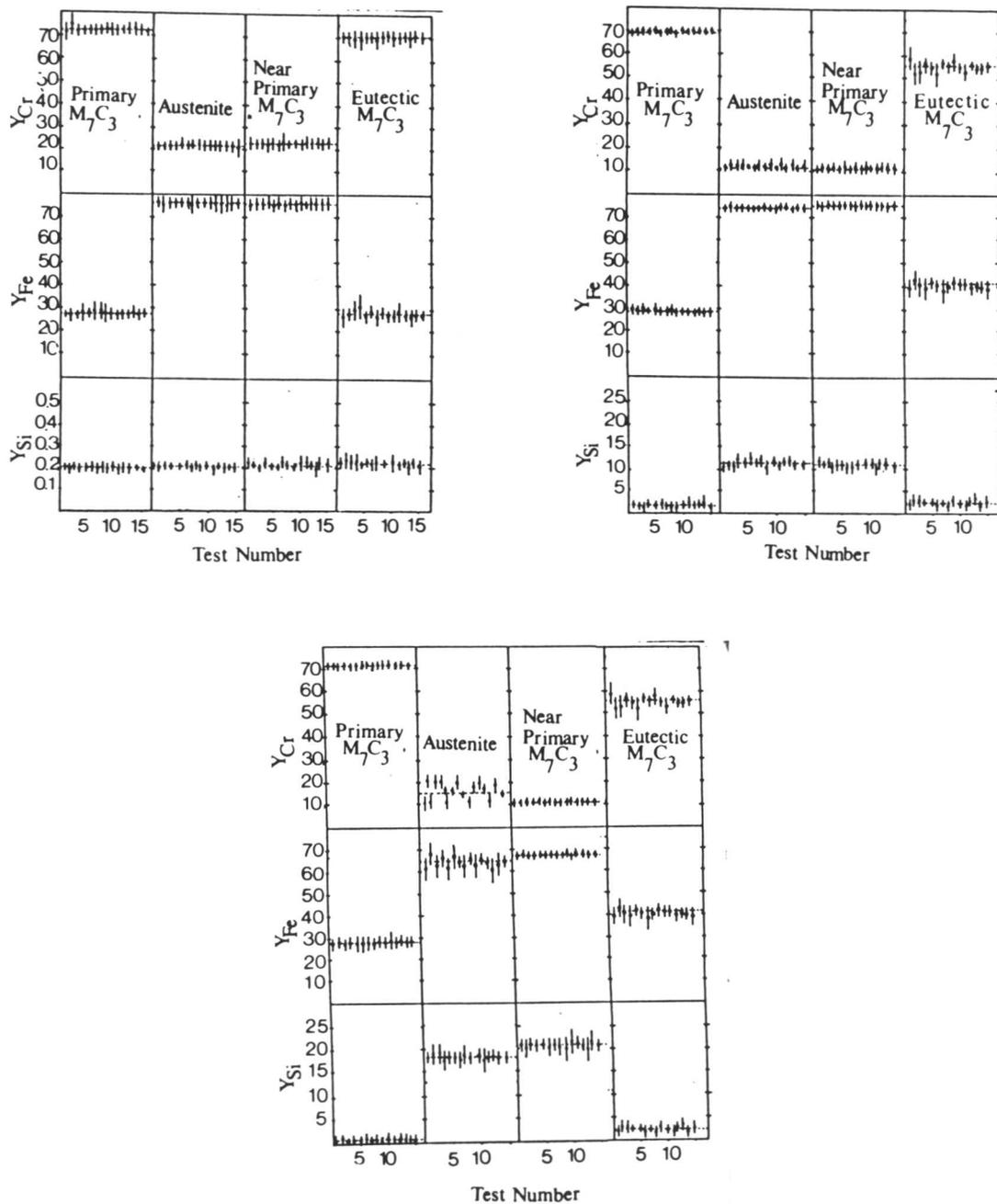
Fig. 7.26: Results of microanalysis experiments carried out in a transmission electron microscope. The dashed lines refer to the average composition. a) Alloy S1; b) Alloy S2; c) Alloy S3.
