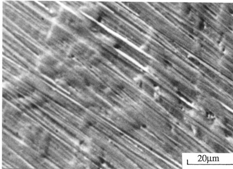
Fig. 7.27: Scanning electron micrograph of the worn surface of alloy S3 after the pin-on-disc abrasion test using SiC abrasives.
