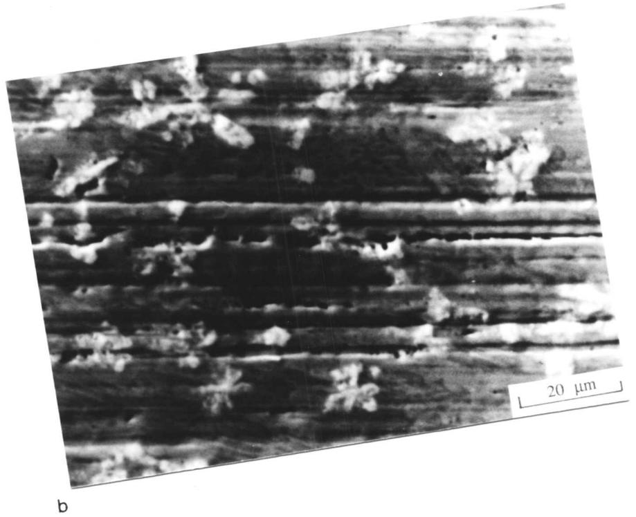
Fig. 8.4: Scanning electron micrographs of the worn surfaces of Alloy 79 after pin-on-disk abrasion tests using SiC (180 mesh) abrasives and a 2kg load. a) low magnification; b) high magnification. It is clear that the abrasives are able to cut the NbC particles. Nonetheless, scratch groove width in NbC is seen to be narrower than in the eutectic areas suggesting that primary NbC improve wear resistance.
