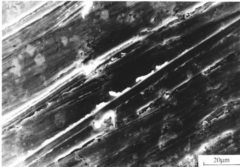
Fig. 8.16: Scanning electron micrograph of the worn surfaces of Alloy 37 after pin-on-disc abrasion test using SiC (180 mesh) abrasives under 2kg load, showing continuous grooves and micromachining process.
