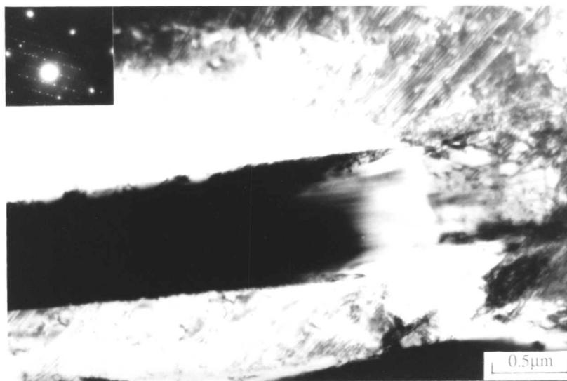
Fig. 8.9: Transmission electron micrograph of the Alloy M4 showing eutectic  $\text{M}_7\text{C}_3$  carbide, in an austenitic matrix. The selected area diffraction pattern from the  $\text{M}_7\text{C}_3$  carbides and austenite is inserted.
