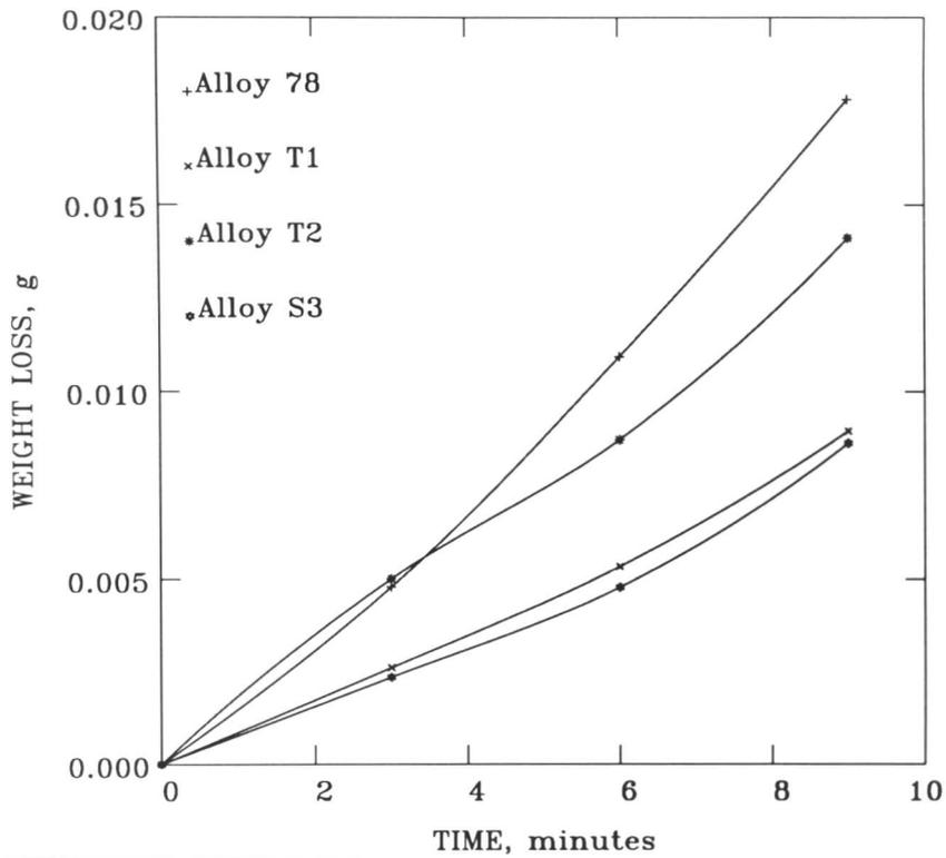
Fig. 7.29: Weight-loss time curves for the alloy 78, T1, T2, and S3 during pin-on-disc abrasion test using SiC abrasives at 1kg.
