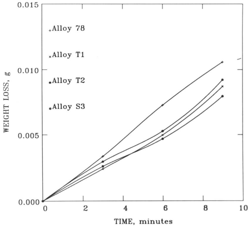
Fig. 7.28: Weight-loss time curves for the alloy 78, T1, T2, and S3 during pin-on-disc abrasion test using Al<sub>2</sub>O<sub>3</sub> abrasives at 450g.
