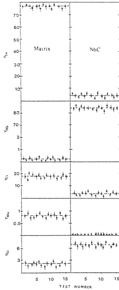
Fig. 8.2: Microanalytical data from Alloy 79 at%. The continuous lines show the average concentrations in each phase. The experiments were carried out using a scanning electron microscopy and energy-dispersive X-ray analysis.
