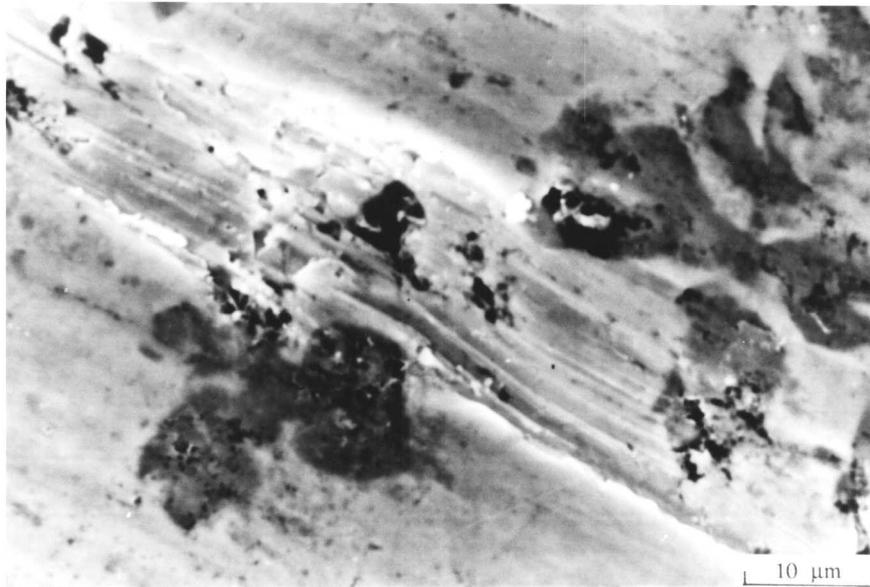
Fig. 8.5: Scanning electron micrograph of the worn surface of Alloy H3, after the pin-on-disc abrasion test using SiC (180 mesh) abrasives and a 2kg load, showing spalling and deformation of TiC due to abrasion.
