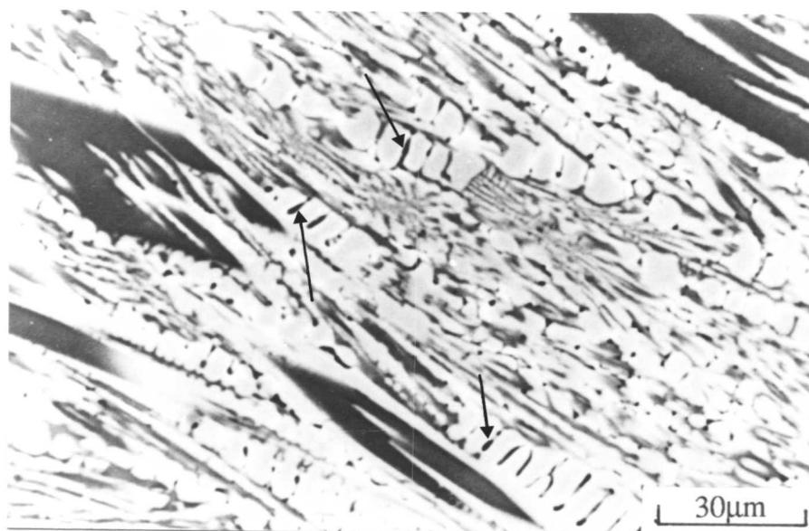
Fig. 8.8: Optical micrograph of alloy M4 (Fe-31.1Cr-3.61C-8.30Mo-0.32Ni-0.24Si-0.20Mn wt%) consisting of primary, and eutectic  $M_7C_3$  carbides with pro-eutectic austenite dendrites. The dark etching regions along the dendrite boundaries are marked by arrows.
