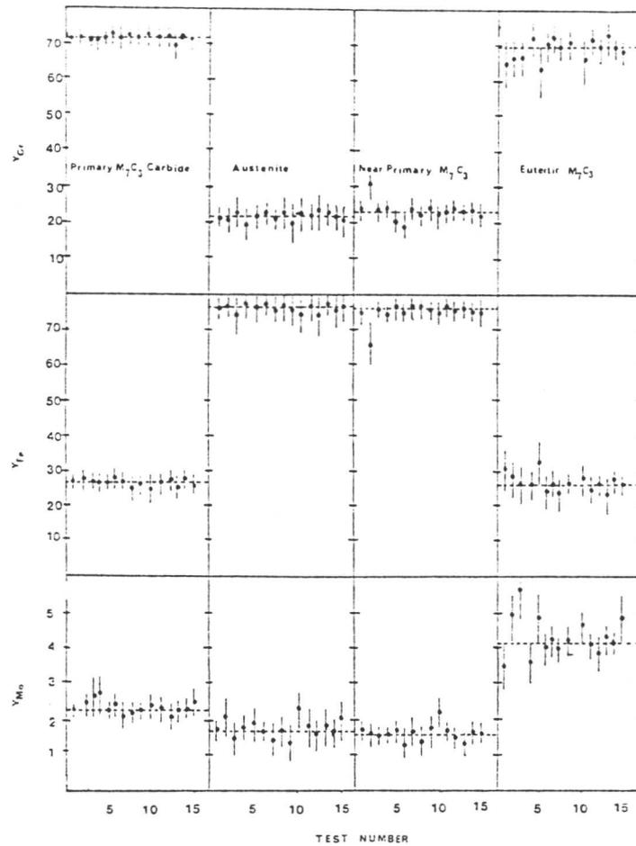
Fig. 8.10: Microanalytical data from Alloy M4 on primary  $M_7C_3$ , near primary  $M_7C_3$ , austenitic matrix, and eutectic  $M_7C_3$  (at%) when the C is not included (continuous lines show the average values in each phase). The experiments were carried out using transmission electron microscopy, and energy-dispersive X-ray analysis. The experiments near the primary carbides (Near P. Carbide) were carried out using scanning electron microscopy.
