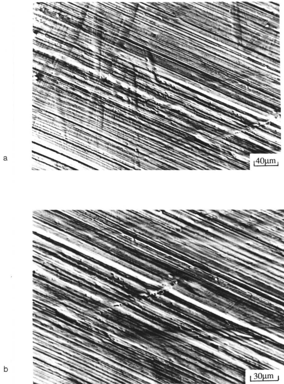
Fig. 7.23: Scanning electron micrographs of the worn surfaces of alloy T1 after the pin-on-disc abrasion test using a) SiC (220 mesh) abrasives at 1kg load; b)  $\text{Al}_2\text{O}_3$  (400 mesh) at 450g, showing that carbides are worn to the same level as the eutectic mixture.
