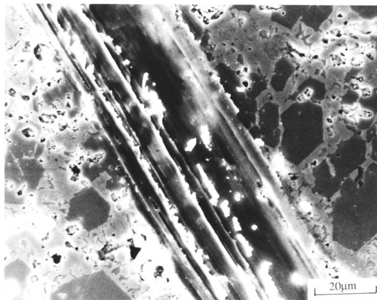
Fig. 8.17: Scanning electron micrograph of the Alloy 37 after single-pass scratch tests using Vickers diamond showing an extensive damage due to micromachining process.
