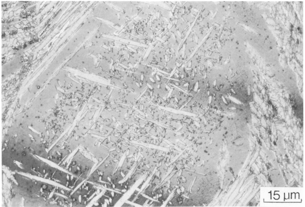
Fig. 5.4.a: Optical micrograph showing the microstructure of the as-welded top layer of alloy BW. The light etching phase is the austenite.
