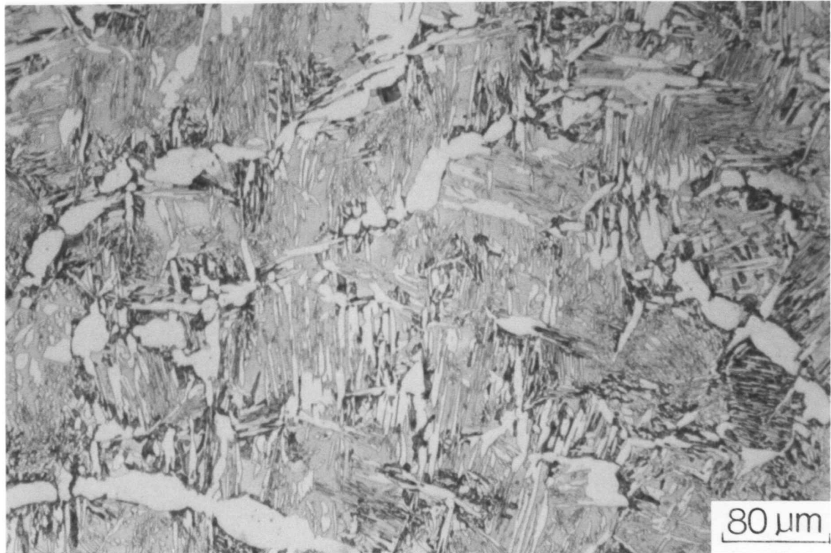
Fig. 6.62: Microstructure of a sample of alloy R4P, after direct isothermal transformation from the \delta + \gamma phase field at 900°C for 15 minutes.
