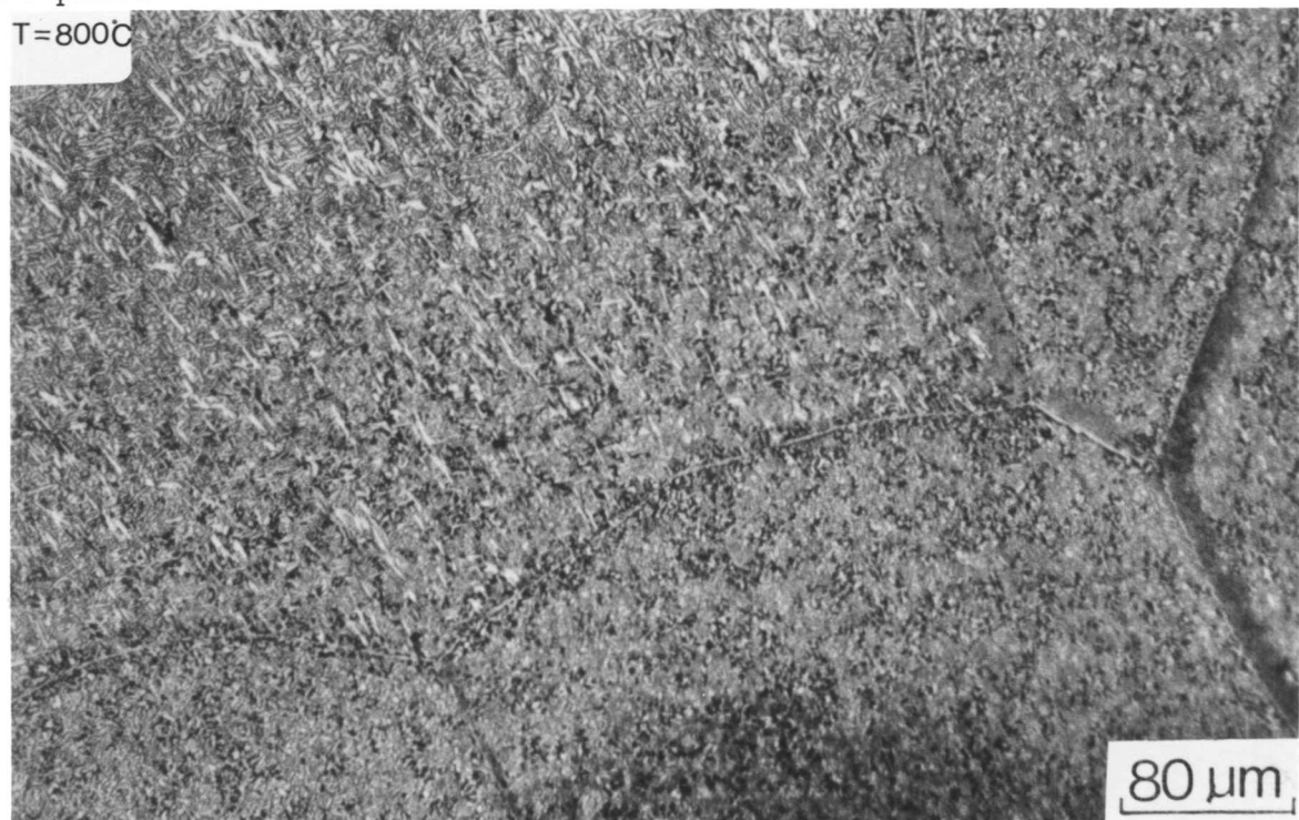
Fig. 6.12: Optical micrograph showing the microstructure of a sample of welded alloy BW, after direct isothermal transformation at 800°C. The light etching phase is austenite. \delta -ferrite is brown and the dark etching phase at the \delta/\gamma boundaries is \sigma phase.
