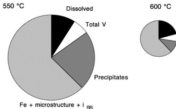
1 Pie charts showing factorisation of  $10^5$  h creep strength of 2.25Cr-Mo steel: diameters of pie charts are scaled to reflect  $10^5$  h strength at appropriate temperature; terms  $i_{SS}$  indicates contributions due to dissolved solutes other than Mo and V (Ref. 6)
