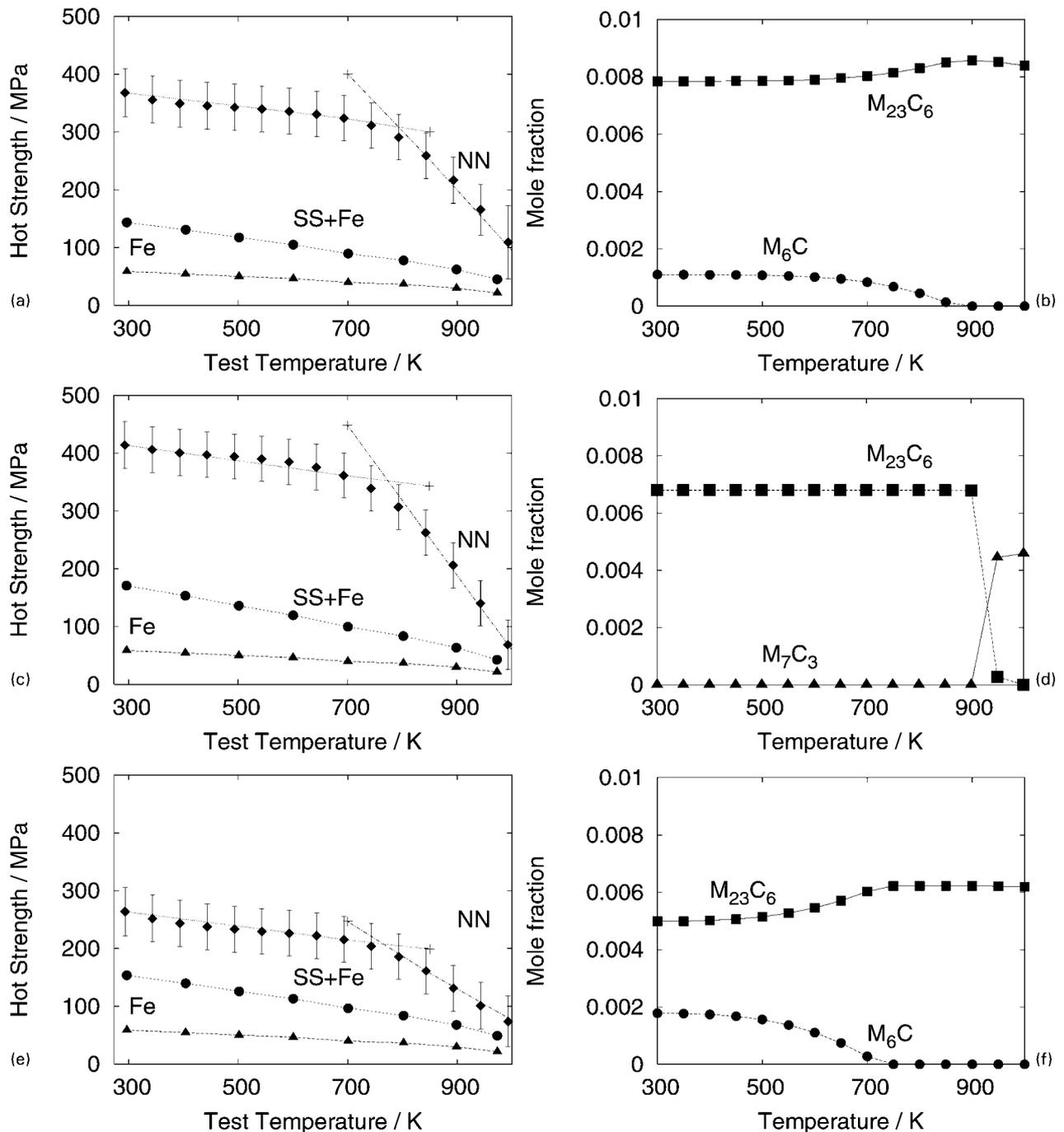
a 2.5%Cr steel: 0.15C-0.18Si-0.63Mn-0.024Ni-2.23Cr-0.97Mo-0.2Cu-0.01Al-0.0083N, 1193 K for 8 h, air cooled, tempered at 993 K for 6 h; b 2.5%Cr steel; c 5%Cr steel: 0.12C-0.33Si-0.56Mn-0.046Ni-5Cr-0.049Mo-0.05Cu-0.066Al-0.017N, 1173 K for 10 min, air cooled, tempered at 1023 K for 120 min; d 5%Cr; e 9Cr-Mo steel: 0.11C-0.59Si-0.41Mn-0.1Ni-9.15Cr-1.05Mo-0.02Cu-0.011Al-0.018N, 1133 K for 30 min, air cooled, tempered at 1033 K for 90 min; f 9Cr-Mo
