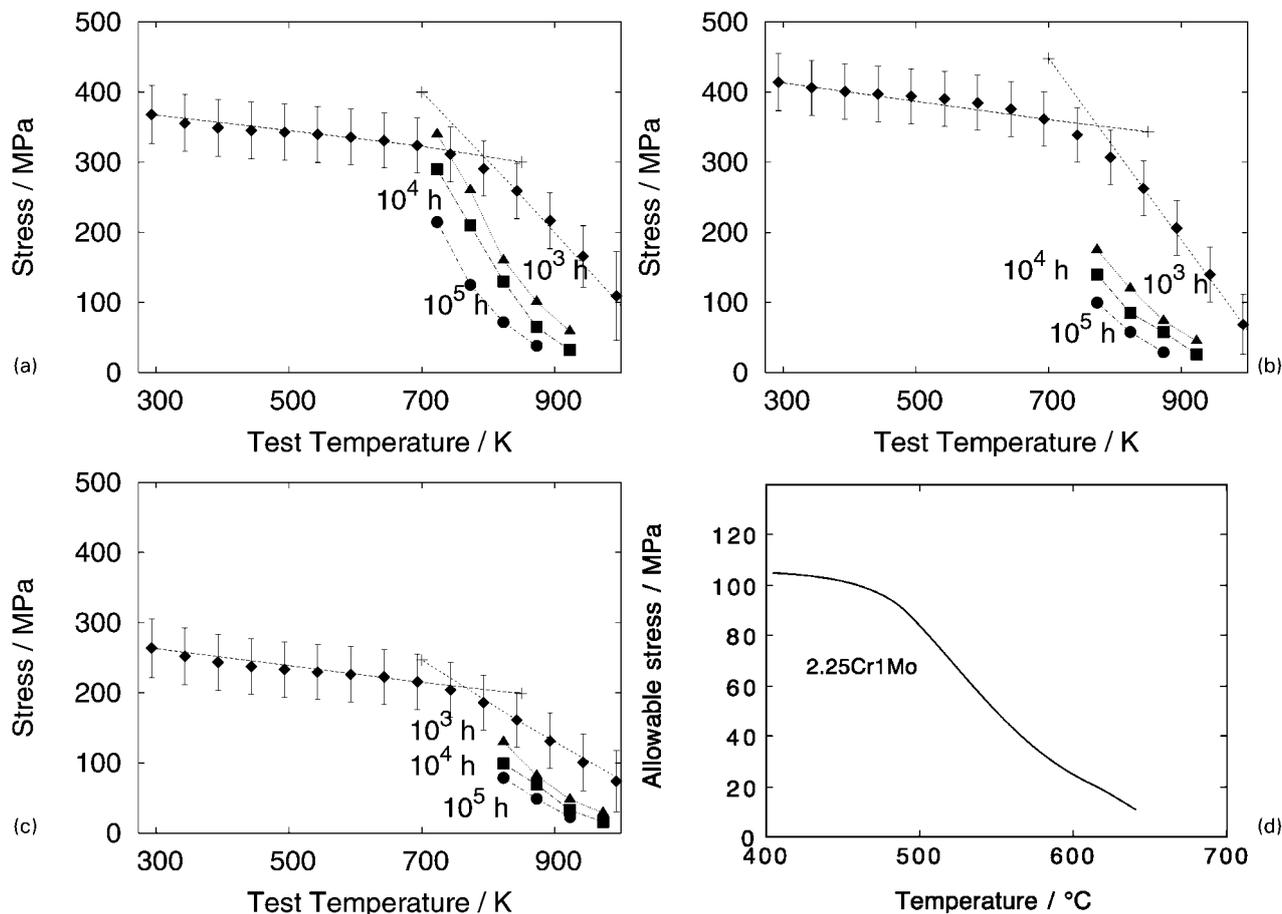
a 2.5Cr-Mo; b 5%Cr; c 9Cr-Mo; d allowable stress for 2.5Cr-Mo steel<sup>29</sup>
