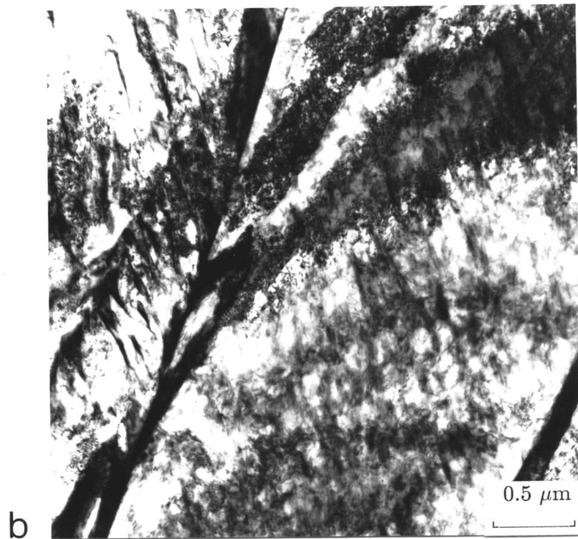
Fig. 4.7: Mixed microstructure of upper and lower bainite obtained by isothermal transformation of homogeneous 300M steel at 320 °C for 60 minutes before quenching to ambient temperature. (a) Bright field image of upper bainite; (b) same sample, but showing lower bainite.
