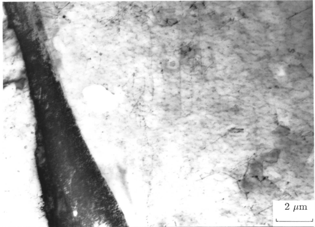
Fig. 7.16: Bright field transmission electron micrograph from a heterogeneous sample of Fe-0.17C-0.35Si-1.38Mn wt. % steel, transformed isothermally to allotriomorphic ferrite at 700 °C for 60 minutes before quenching to ambient temperature. Shows allotriomorphic ferrite and residual austenite.
