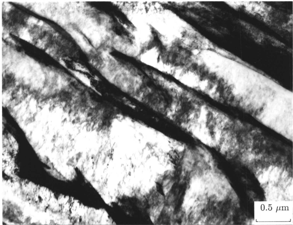
Fig. 8.15: Bright field transmission electron micrograph showing upper bainite in a heterogeneous sample of 'US24' steel.
