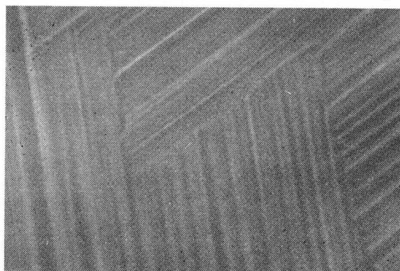
13 Surface relief markings produced by transformation of a cubic single crystal of a Co-30.3%Ni alloy, to illustrate formation of a jagged interface 28 ×1600
