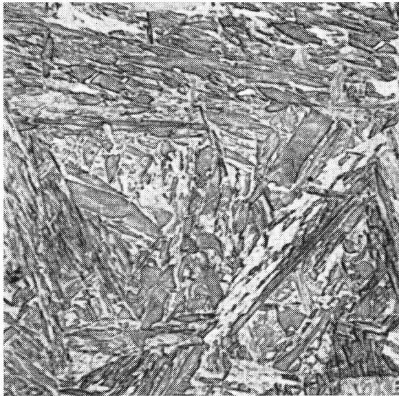
E Acicular plate-like martensite in 0.21%C-2%Mn alloy; found to be practically untwinned when examined in the electron microscope; hardness about 450 HV10 \times 1000
