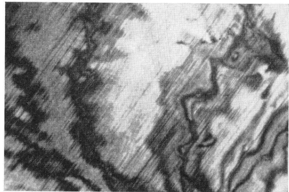
6 Interior of a \beta'_1 -martensite plate with striations due to stacking faults parallel to the electron beam; Cu-13.7 at-% Sn; transmission electron micrograph \times 70000
