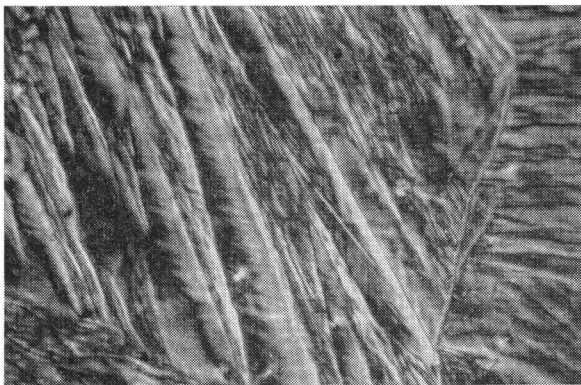
B Fe-18%Ni alloy, pre-polished and transformed in vacuum to massive martensite \times 750
