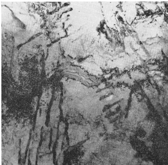
8 Upper bainite formed at 420°C in the 0.96% C steel ×30000
