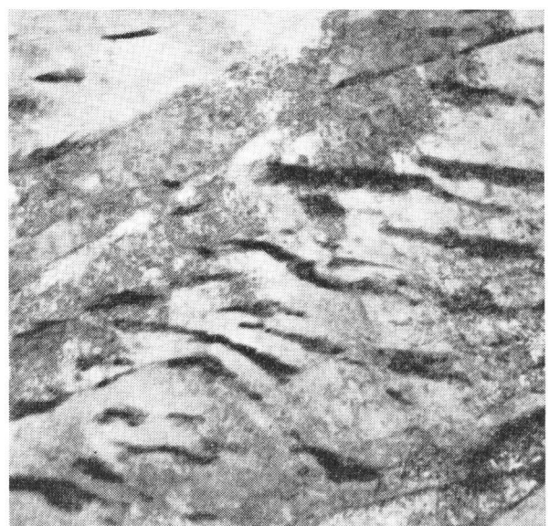
14 Upper bainite formed at 480°C in the 0.39% C steel \times 30000
