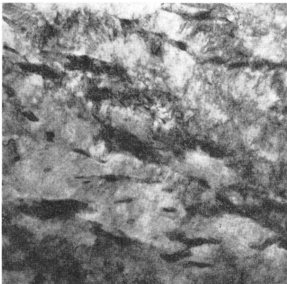
12 Upper bainite formed at 420°C in the 0.39% C steel \times 60000
