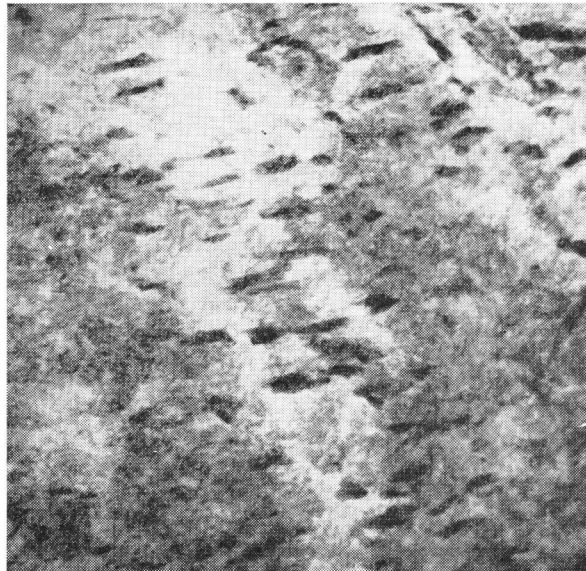
10 Upper bainite formed at 420°C in the 0.58% C steel ×30000
