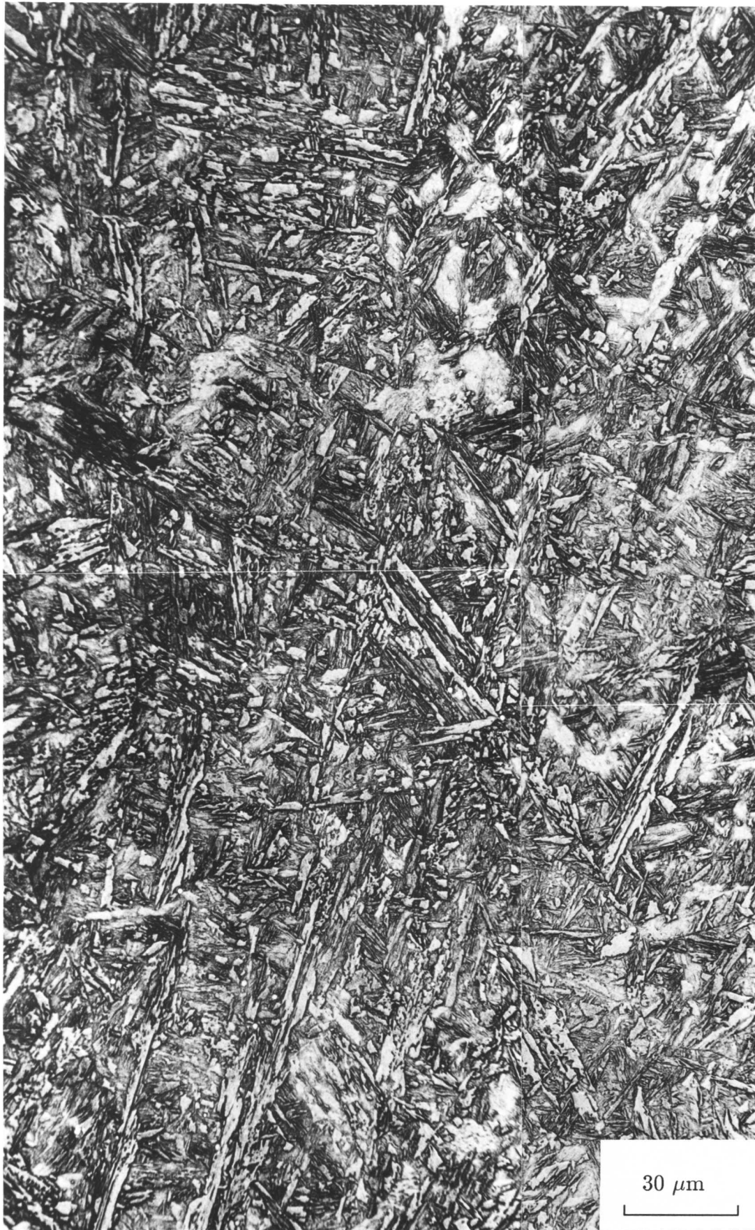
Figure 9.9 The microstructure of alloy 115 isothermally transformed for five minutes at 470°C after austenitisation for 1 minute at 1350°C. The acicular ferrite fraction is very low, therefore sheaf formation is pronounced (arrowed).
