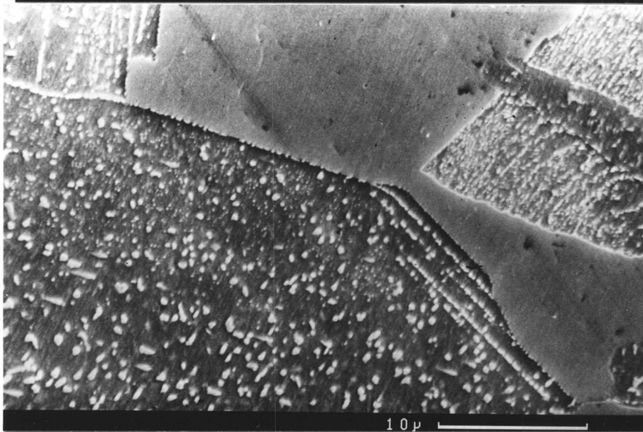
Fig. 4.13(a) to (c) Showing variation in the band spacing. Random carbide precipitation is also visible.
