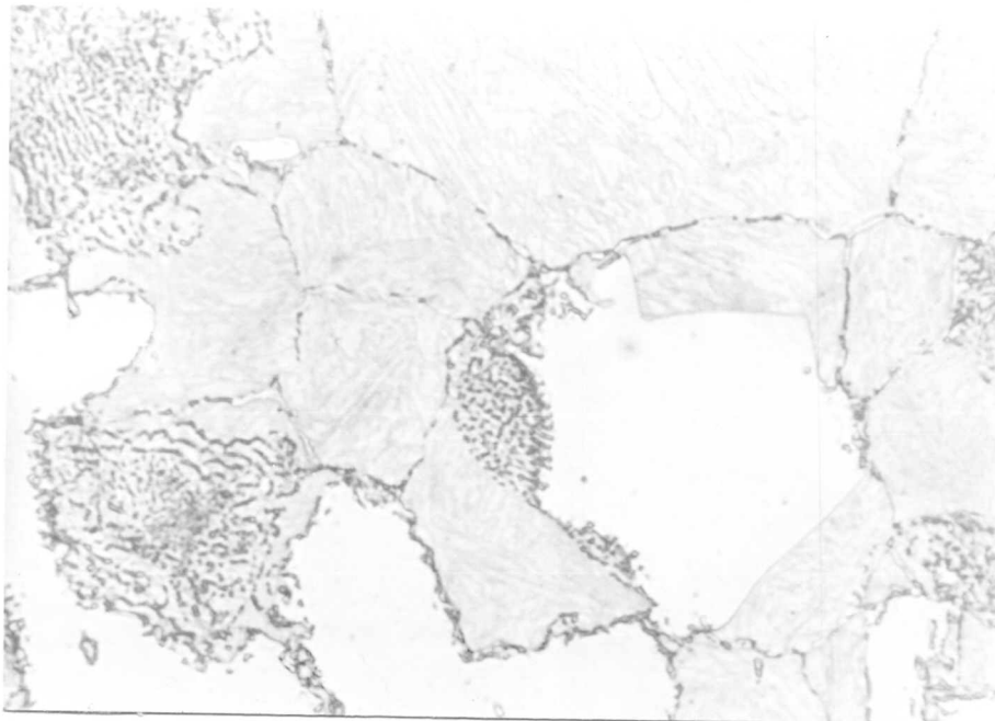
Figure 5.4a: With increasing time of transformation the carbides grew in austenite (850°C/80 Min).
