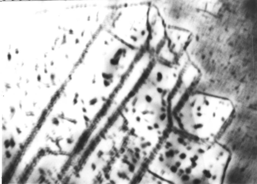
Fig. 4.32 to 4.34: Microstructure developed by double step quenching. 2μ
