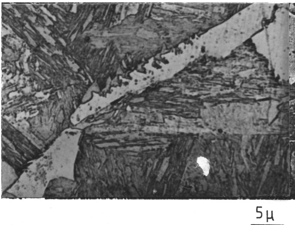
Figure 8.28: Showing evidence of interface pinning. (610°C/20 min).
