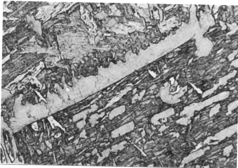
Figure 8.12: Grain-boundary allotriomorphic ferrite growing along the prior austenite grain-boundary. (750°C/40 sec).
