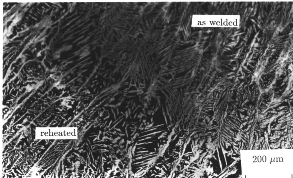
Figure 4.19. Light micrograph shows referritised region in reheated weld metal A219.
