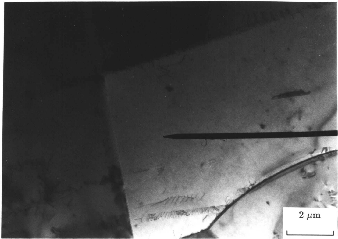
Figure 3.20. TEM micrograph showing the microstructure of rolled duplex stainless steel alloy IC378. The electron diffraction pattern of the pointed phase (Figure 3.21) confirms that its crystal structure is b.c.c. and the TEM EDX microanalysis of this phase (Table 3.6) shows the partition of ferrite stabilisers in this phase confirming it is ferrite.
