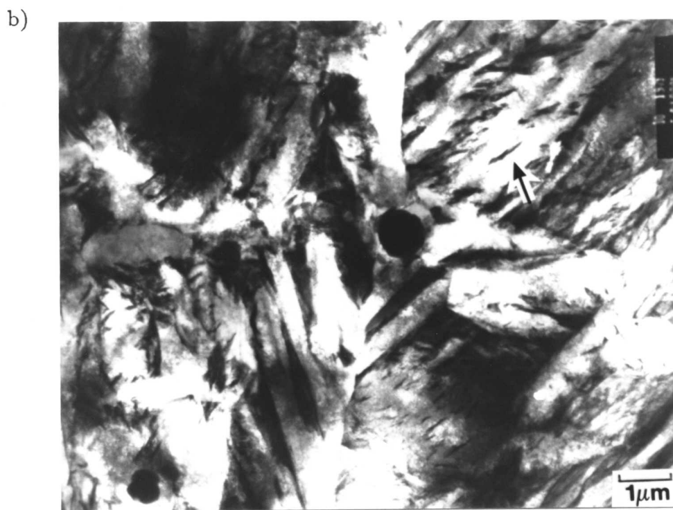
Figures 10.7a and b: Classical bainite subunits nucleated at the prior austenite grain boundaries of Weld 10.1. The grey phase between the subunits in Figure 7a is likely to be retained austenite. Lower bainitic carbides (arrowed) may be seen within the ferrite, towards the top right of Figure 7b.
