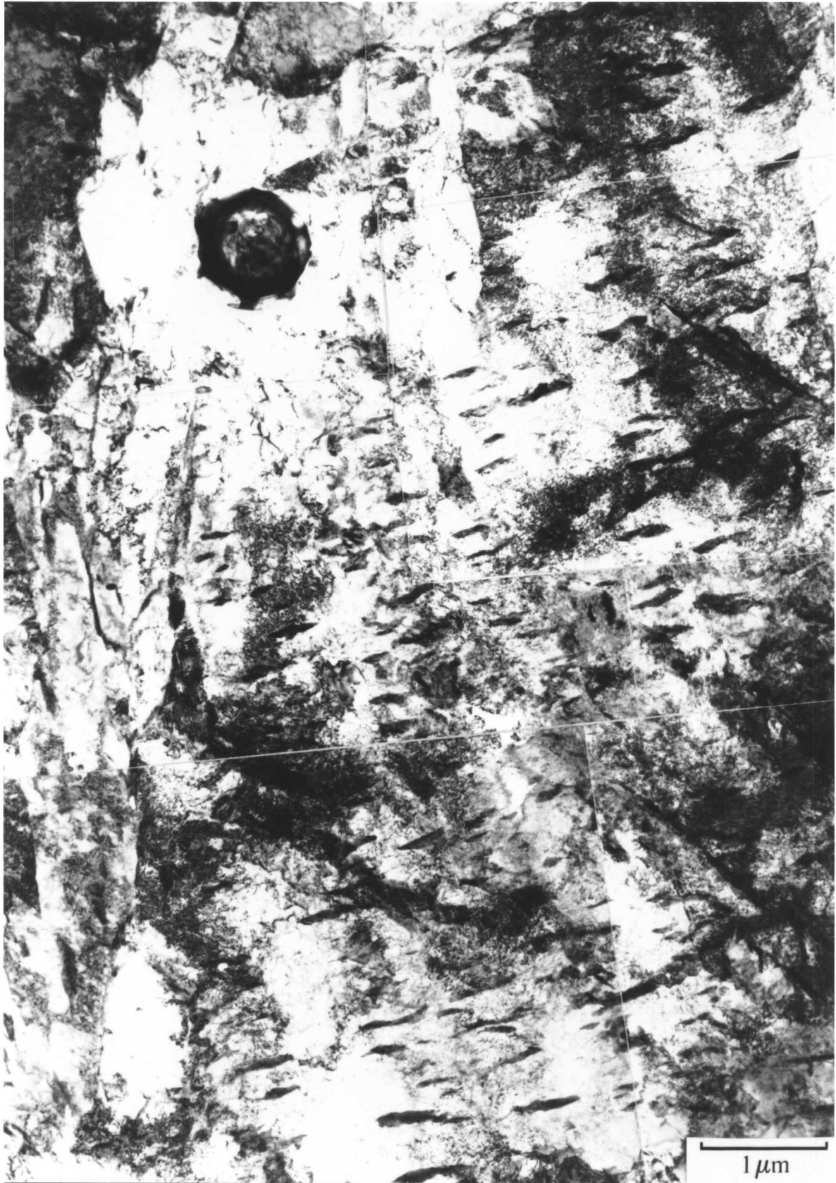
Figure 10.10: Photo-montage of the microstructure of Weld 10.1 within the columnar grains showing classical lower bainitic microstructure.
