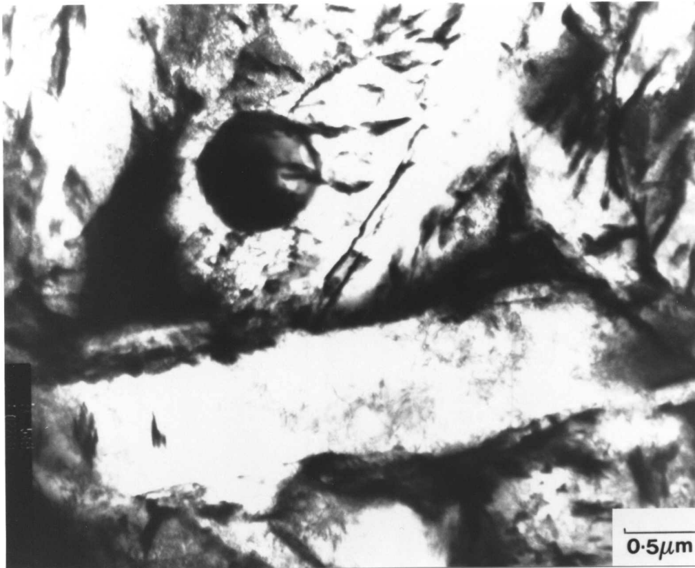
Figure 10.14: Micrograph quintessentialising the microstructure of Weld 10.1. The micrograph shows a spherical oxide inclusion surrounded by bainitic ferrite. Subunits of upper and lower bainite may both be seen. Note the high dislocation density within the upper bainite.
