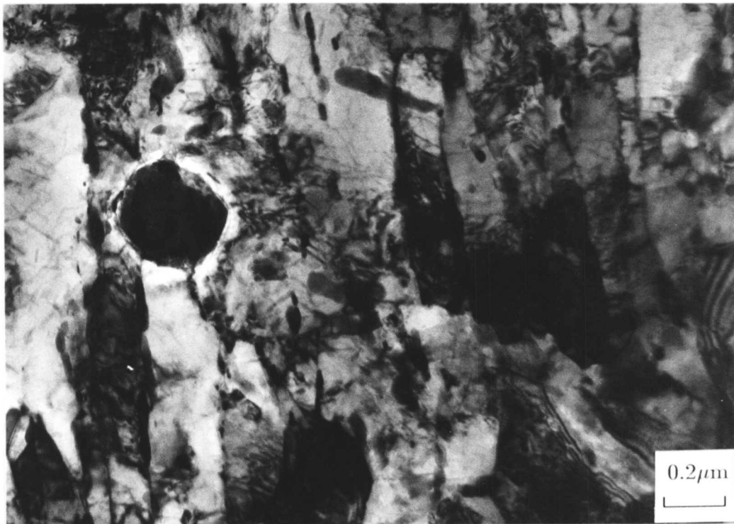
Figure 5.32: A similar upper bainitic region; a large MnS inclusion can be seen within the microstructure, and there is extensive cementite precipitation on the plate boundaries and Mo_2C within the sheaves.
