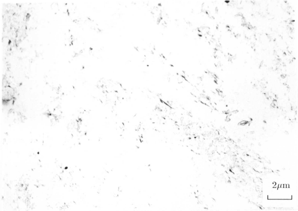
Figure 5.23: Carbon extraction replica from the fully bainitic specimen tempered for 10 minutes at 565°C showing that cementite has begun to precipitate, in particular in between and parallel to the plates of upper bainite.
