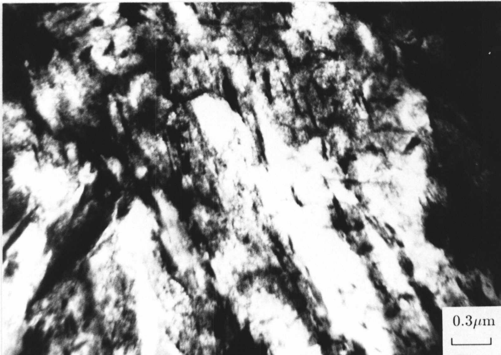
Figure 5.24: Transmission electron micrograph from a thin foil specimen from the fully bainitic specimen tempered for 10 minutes at 565°C showing a plate of tempered martensite containing cementite in three distinct orientations.
