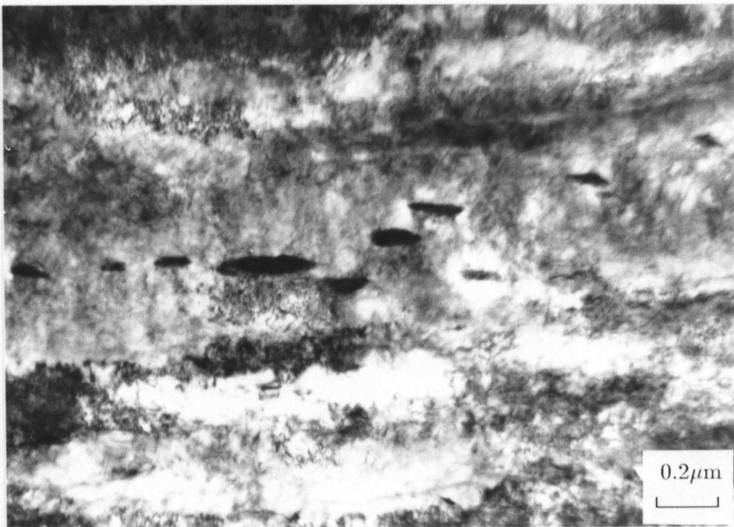
Figure 5.12: High magnification image of a lower bainite plate in this case showing cementite precipitation parallel to the axis of the plate.
