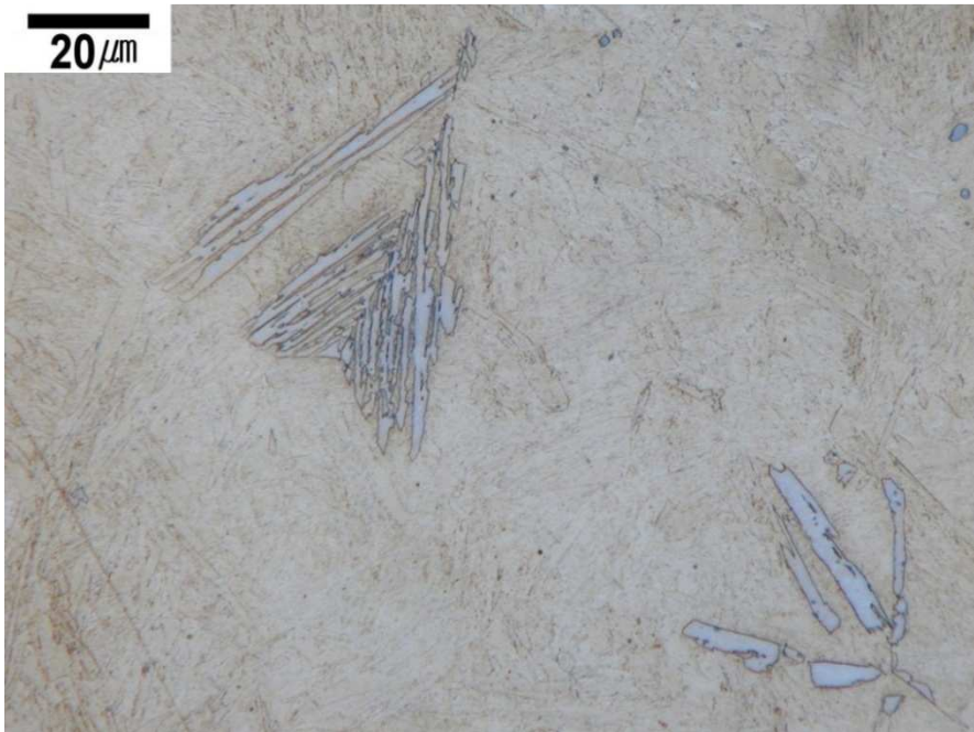
(c) 5Ni alloy. Isothermally transformed at 460 °C. Small fraction of bainite was formed.
