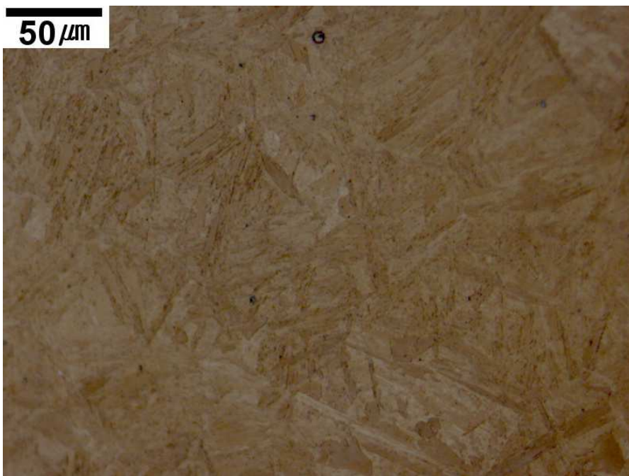
(b) 6Ni alloy. Isothermally transformed at 310 °C for 3 h. No bainite, fully martensitic.
