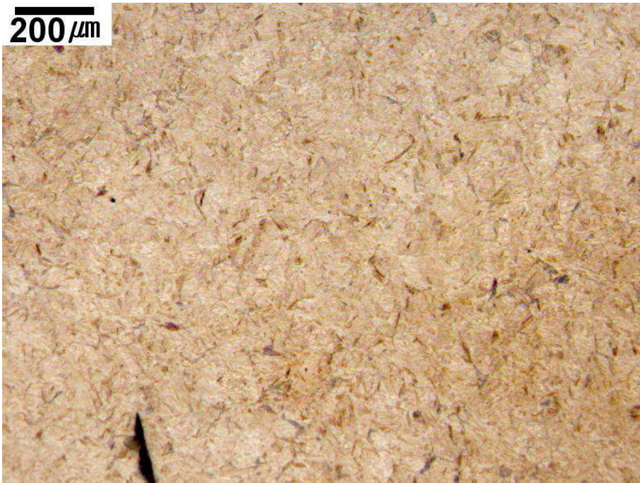
(a) 4Ni alloy. Quenched sample for reference. Fully martensitic.
