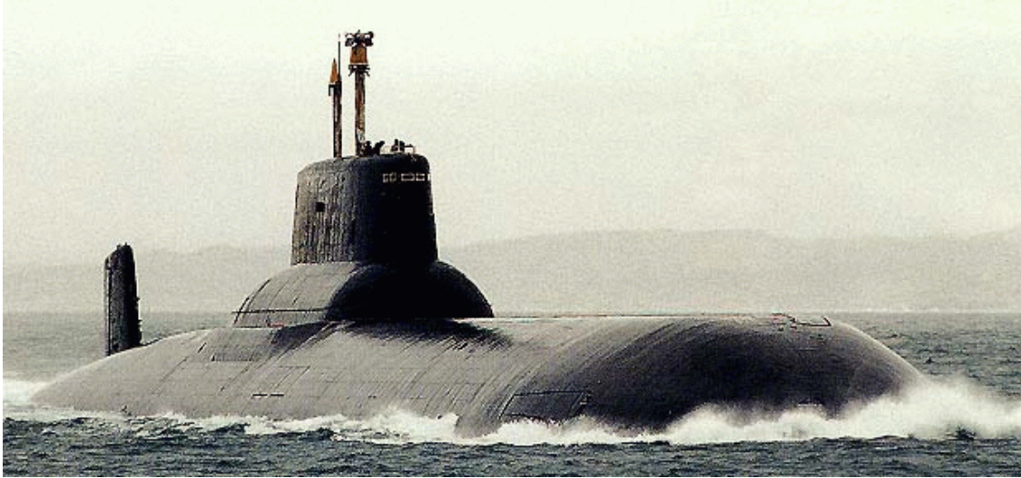
Figure 1.1: A typical application — at 172 m long, the Russian Navy’s latest Typhoon class nuclear submarines are the largest ever constructed [1].
