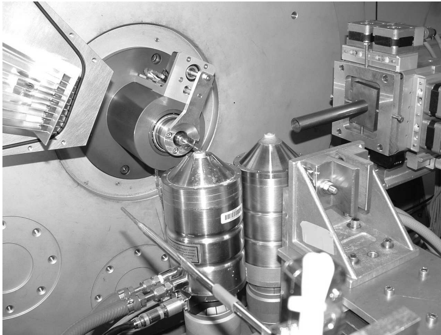
Figure 3. Sample assembly mounted on the ID31 diffractometer hot-air blowers positioned underneath.
