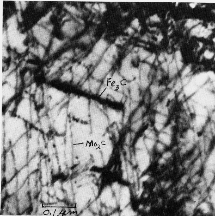
Figure 14. Nucleation of \text{Mo}_2\text{C} Particles at Dislocations and Dissolution of Cementite in 10Ni-8Co-2Cr-0.12C Steel Tempered 30h at 480C [5].
