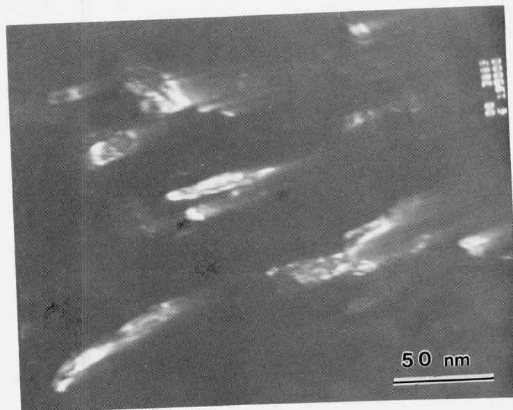
Fig. 16 TEM micrograph showing a Bright/Dark field image of intralath austenite particles in AF-1410 steel. Direct-nucleated austenite treatment ( 600^{\circ}\text{C}/15\text{min}+510^{\circ}\text{C}/8\text{h} ).
