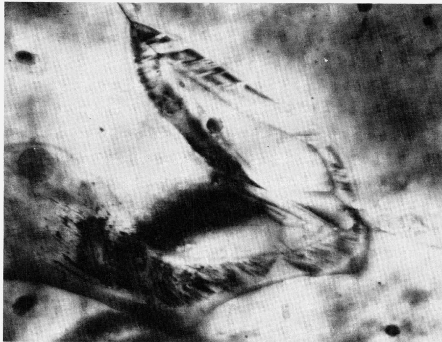
Fig. 13 STEM micrograph (bright field image) of Alloy B (CRT series) after intercritical treatment at 740°C for 100 seconds. A pool of austenite has transformed to martensite at the grain boundary.
