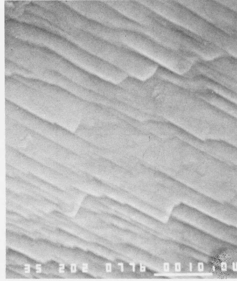
Fig. 6. The small faceted fracture area of the \Sigma 11 bicrystal. (1123 K, 24 hrs. + 773 K, 24 hrs in Bi vapor)
