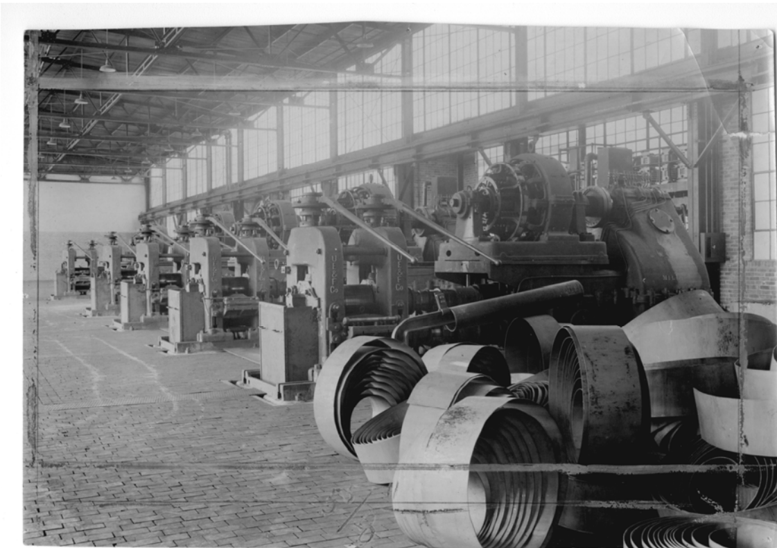
Figure 2. The continuous wide hot strip mill finishing train of Columbia Steel, Butler, Pennsylvania with United Engineering and Foundry Company four high stands and Messinger roller bearings – Townsend and Naugle appear to be standing on the extreme left of the picture (courtesy of the Hagley Museum and Library, Delaware)
