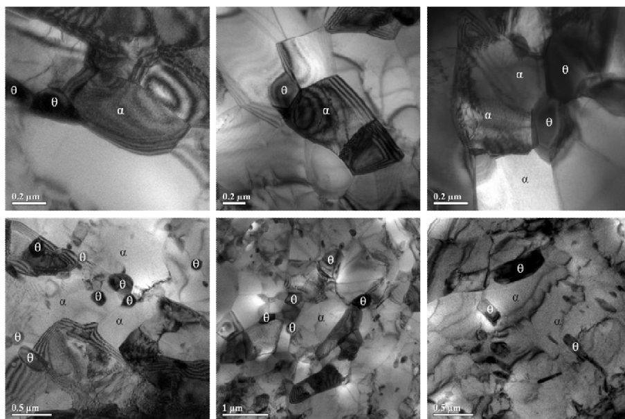
Fig. IV.8 Bright field image of 1-400h indicating positions where the Mn content was determined using EDS. Ferrite is indicated as \alpha and cementite, \theta .
