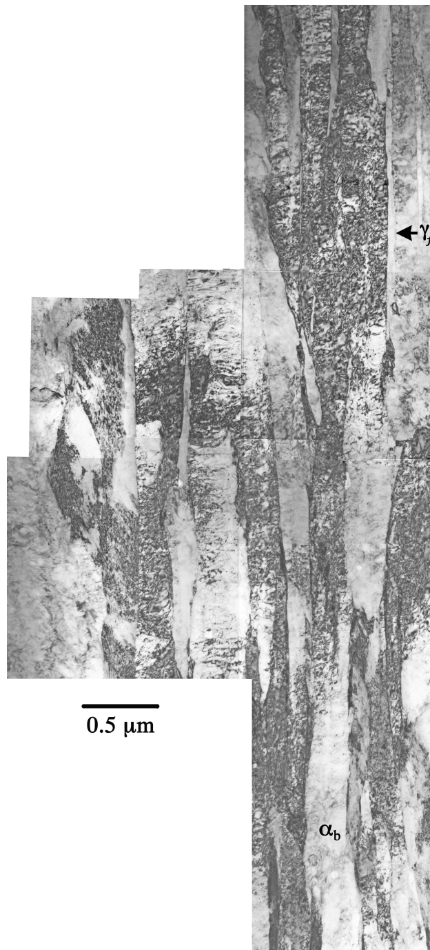
Figure 1.2: Transmission electron micrograph showing bainite ferrite ( \alpha_b ) with retained austenite films ( \gamma_f ) entrapped between the ferrite plates (From present work).
