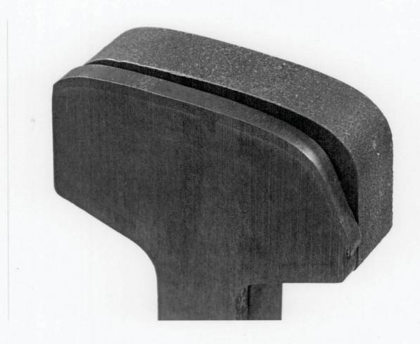
Figure 1.1 A comparison between new and worn rails. This shows the typical form of severe gauge face wear that occurs on outer rails, installed in tight curves, on the British Rail network [Print kindly donated by British Rail Research].
