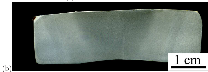
Figure 5.15: As-etched ND-TD surface of the weld from the pipe with 14.8 mm wall-thickness. (a) As-welded. (b) Heat-treated.
