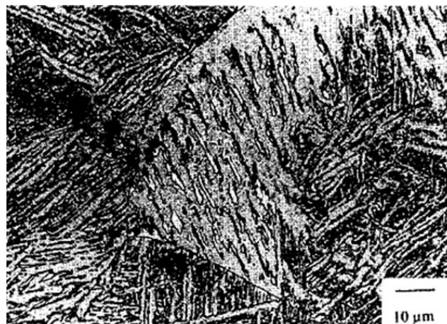
Figure 2.8. Light microscopy image of the heat-affected zone of C-Mn steel in welding, the carbides are black, the M/A constituents white, and the ferrite gray. Reproduced from [Alé et al. , 1996] with permission from Elsevier.
