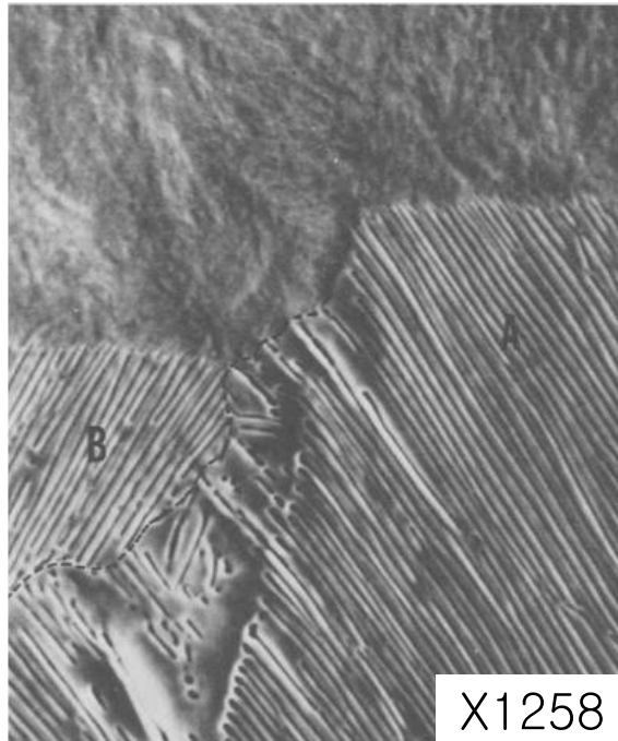
Figure 4: A longitudinal section of forced velocity pearlite at a quenched interface with a prior austenite grain boundary separating pearlite colonies A and B [37].
