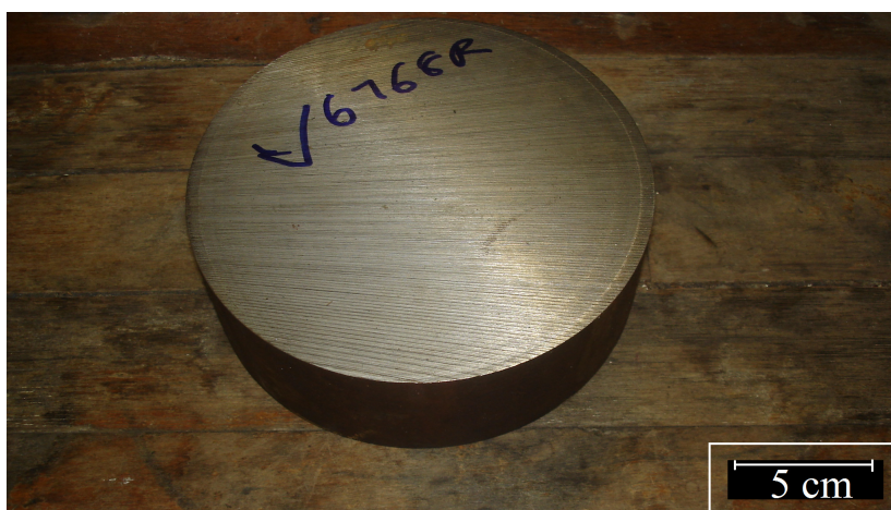
Figure 3.1: A section of the shaft material in as-received condition.
