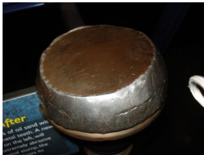
Figure 2.4: Wear of the hardfacing layer on the tooth. Courtesy H. K. D. H. Bhadeshia.
