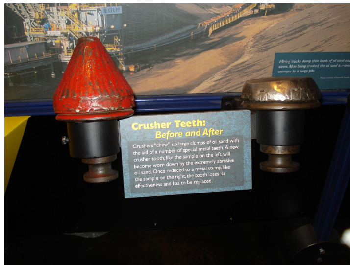
Figure 2.3: The tooth on the left is at the beginning and the one at the right after it has been worn down by abrasive oil sands. Courtesy H. K. D. H. Bhadeshia.
