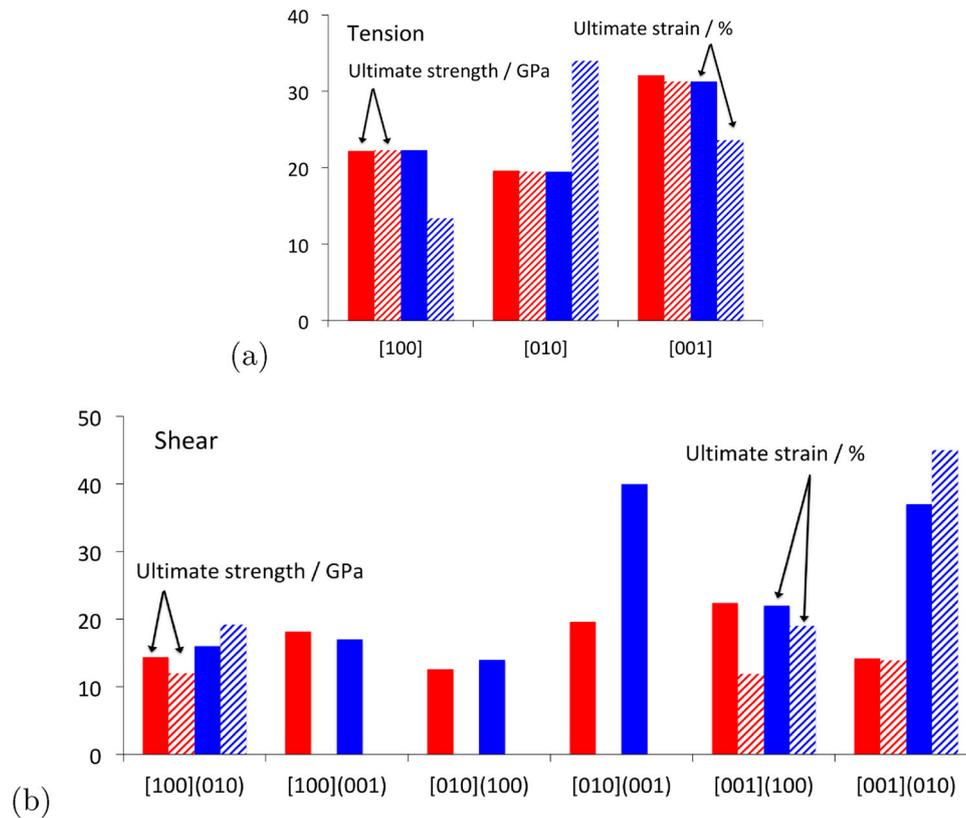
**Figure 20.** Calculated ideal values of ultimate strength at corresponding engineering strains for perfect crystals of cementite. (a) Tensile deformation along crystallographic axes parallel to the cell axes. (b) Shears on the planes and directions indicated. Uniform colour indicates data from Garvik et al. [51] whereas the cross-hatched bars are from Jiang and Srinivasan [37].
