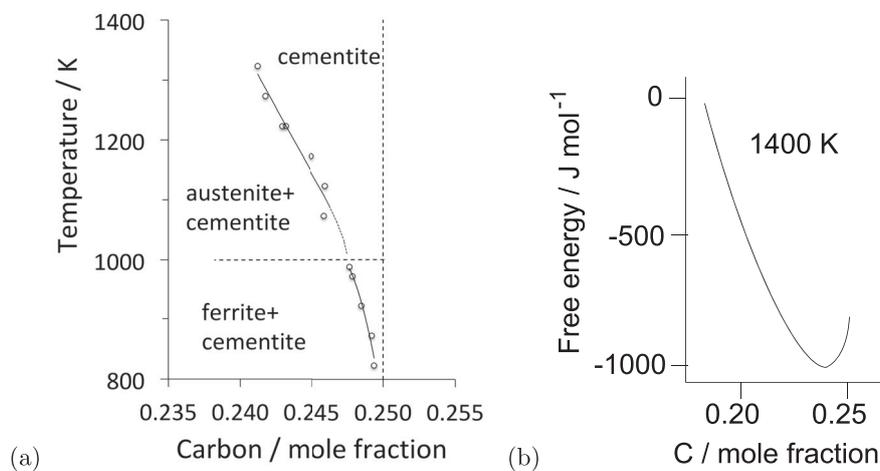
**Figure 3.** (a) The composition of cementite that is in equilibrium with austenite or with ferrite in an Fe-C alloy. The data are due to Leineweber et al. [17], determined by measuring the lattice parameters of cementite following quenching from the appropriate temperature. (b) Free energy curve of cementite as a function of chemical composition (referred to  $\gamma$ -Fe and graphite). After Gohring et al. [18].
