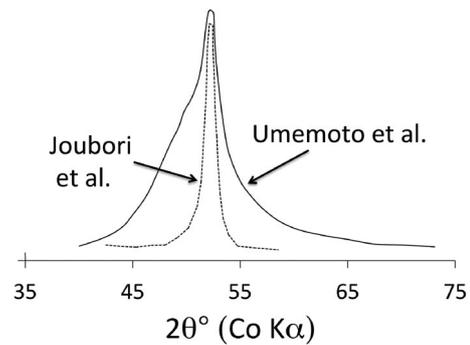
**Figure 17.** A comparison of the  $\{110\}_0$  X-ray peaks from the experiments of Umemoto et al. [113] and Joubouri et al. [118] – the latter has been corrected to the Co  $K_\alpha$  wavelength to permit the comparison.
