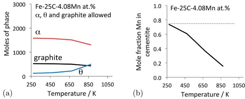
**Figure 23.** Phase diagram calculations for 100 kg total weight, using MTDATA [11] and the SGTE thermodynamic database. Fe-25C-4.08Mn at.%, permitting cementite, graphite and ferrite to co-exist. (a) Equilibrium phase mixture as a function of temperature. (b) The equilibrium manganese concentration in cementite for the calculations presented in (a).
