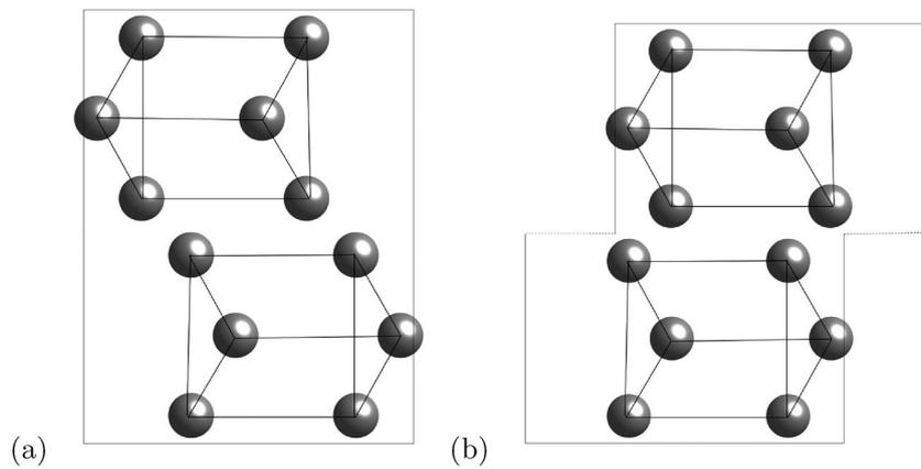
**Figure 7.** Creation of a stacking fault on  $(010)_0$  by a partial displacement parallel to  $[100]_0$  that does not recreate the lattice. Carbon atoms have been omitted for clarity. (a) Unfaulted structure. (b) Faulted structure. Adapted from [48].
