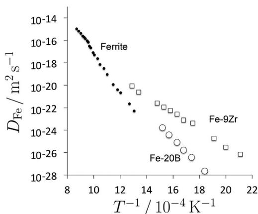
**Figure 31.**  $^{59}\text{Fe}$  tracer diffusion coefficients in Fe–Zr and Fe–B glassy metals in the relaxed state. Self-diffusion data for iron in ferrite are included from [194,195], for comparison purposes. Selected data on the amorphous alloys from Horvath et al. [193].
