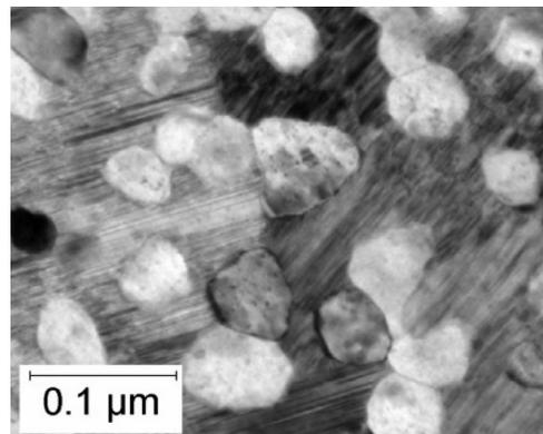
**Figure 30.** Cementite (majority phase, containing planar faults) and equiaxed ferrite, crystallised from metallic glass films of composition Fe-13.6C at.% by heat treatment at 300°C for 3 h. Reproduced from Fillon et al. [192] with permission from Elsevier.
