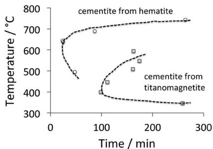
**Figure 29.** Time, temperature and 50% transformation diagrams for the decomposition of cementite into elemental iron and carbon. In one case, the cementite is made by carburising haematite ore ( $\text{Fe}_2\text{O}_3$ ), and in the other by similarly carburising titanomagnetite ( $\text{Fe}_{(1-x)}\text{Ti}_x\text{O}_4$ ). Selected data from Longbottom et al. [189].
