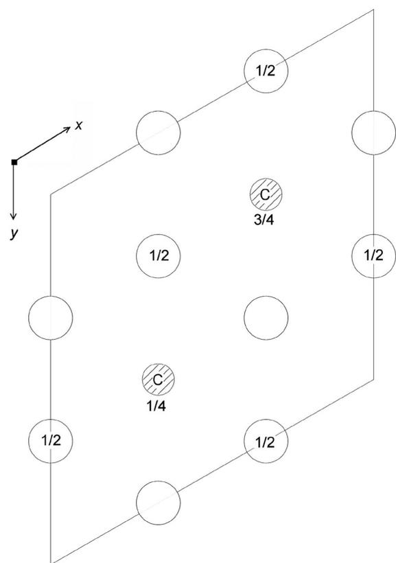
**Figure 8.** Projection of the possible crystal structure of the hexagonal form of cementite, using the parameters and symmetry proposed by Nagakura [57]. The fractional  $z$ -coordinates of atoms not located at  $z=0,1$  are marked. The carbon atoms (hatched) are located in a third of the octahedral interstices formed by the iron atoms.
