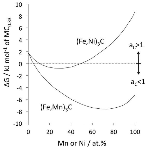
**Figure 24.** The free energy of formation associated with the reaction  $\text{M} + \frac{1}{3}\text{C} \rightarrow \text{M}_3\text{C}$  occurring at 650°C, as a function of the manganese or nickel concentrations. Adapted from Grabke et al. [156].
