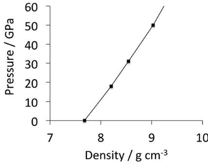
**Figure 15.** Experimentally determined plot of pressure versus density for polycrystalline cementite. The gradient increases with density, indicating an increase in the bulk modulus with pressure. Data from Fiquet et al. [101].
