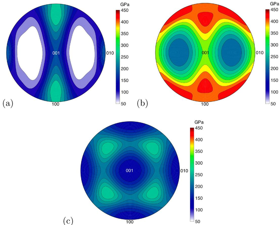
**Figure 14.** Stereographic projections showing the variation of calculated single-crystal elastic moduli as a function of orientation, for the setting  $Pnma$ . (a)  $Fe_3C$  [96]. (b)  $Mn_3C$ , using data from [96] and lattice parameters from [100]. (c) Corresponding data for body-centred cubic iron. Plots courtesy of Shaumik Lenka.
