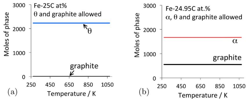
**Figure 2.** Phase diagram calculations for 100 kg total weight, using MTDATA [11] and the SGTE thermodynamic database. (a) Fe-25C at.-%, permitting only cementite and graphite to coexist. (b) The average carbon concentration is reduced slightly to allow ferrite to appear, in which case the most stable mixture becomes that of ferrite and graphite.
