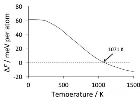
**Figure 28.** The formation energy  $\Delta F$  of cementite for the reaction  $F_{\text{Fe}_3\text{C}} - [3F_{\text{Fe}} + F_{\text{graphite}}]/4$ . Data from CALPHAD assessment by Hallstedt et al. [172]. A negative value implies that cementite becomes stable relative to the mixture of  $\alpha$  and graphite.
