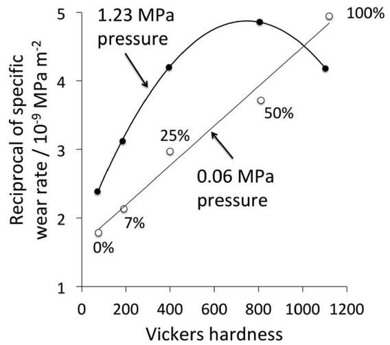
**Figure 22.** Data from the abrasion of a pin made out of the material of interest, against an alumina disc. After Sasaki et al. [146].
