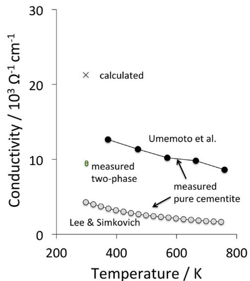
**Figure 19.** The data on pure cementite are from [113,132], the calculated datum from [69] and the measurements of mixed microstructures, extrapolated to single-phase cementite, from [133].
