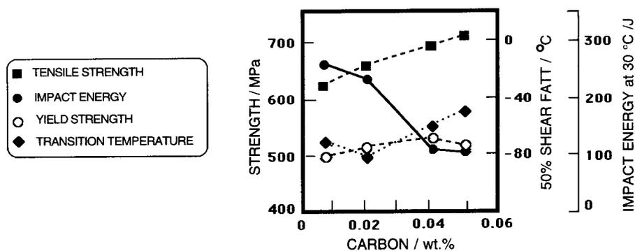
Fig. 8: Variations in mechanical properties as a function of carbon concentration in thermomechanically processed ultra-low-carbon steels [21]. The fracture assessed impact transition temperature (FATT) begins to increase as the carbon concentration falls below about 0.02 wt.%.
