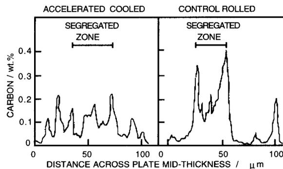
Fig. 7: Distribution of carbon concentration in the segregated zone for conventional control-rolled and rapidly cooled steel plates [19].
