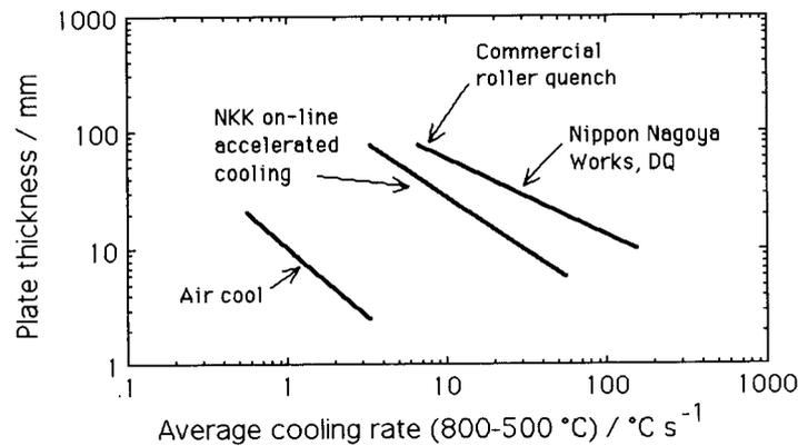
Fig. 3: An illustration of the average cooling rates associated with the manufacture of steels for structural applications [8].
