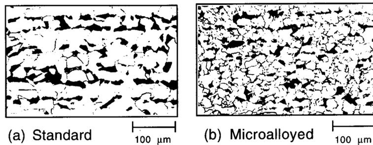
Fig. 1: Optical micrographs of banded ferrite-pearlite microstructures in (a) standard, (b) niobium microalloyed structural steel.
