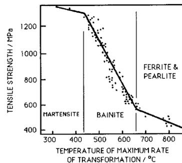
Fig. 2: Variation in the tensile strength of structural steels as a function of the temperature at which the rate of transformation is greatest during continuous cooling heat treatment [7].
