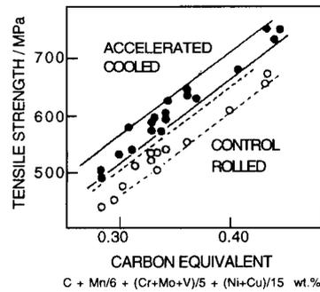
Fig. 6: Relationship between the carbon equivalent and tensile strength for conventionally produced control-rolled steels (CR) and accelerated cooled steels (AC); the latter have a mixed microstructure of ferrite and bainite [13].
