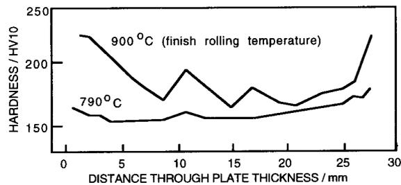
Fig. 4: The effect of the temperature at which rolling is completed, on the variation in hardness of a Fe-0.16C-0.63Mn wt% accelerated cooled steel containing bainite [15].
