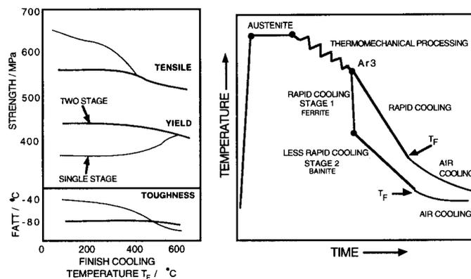
Fig. 5: (a) The relationship between the tensile and yield strength, and toughness of accelerated cooled steels as a function of the temperature at which the forced cooled is stopped, for the single and double stage processes. (b) Schematic illustration of the thermomechanical cycles associated with the two-stage accelerated cooling process [17].
