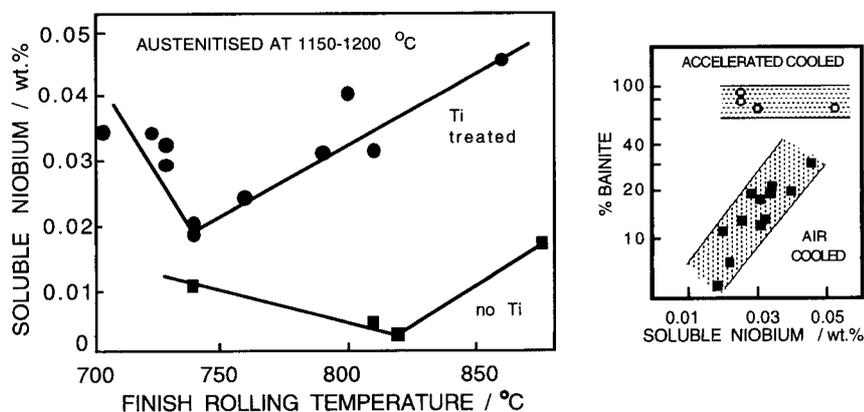
Fig. 9: Soluble niobium in ULCB steel [21]. (a) Variation in the soluble niobium concentration as a function of the finish rolling temperature; (b) variation in microstructure as a function of the finish rolling temperature.
