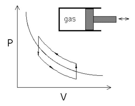
Fig. 1: The curve represents the variation in pressure within the cylinder as the volume of the ideal gas is altered by positioning the frictionless piston. The cycle represents the dissipation of energy when the motion of the piston causes friction.
