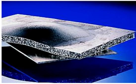
**Figure 7** *Metal foam of high stiffness and low-density ideal for sandwich construction [9].*
