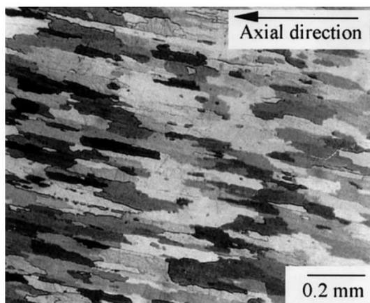
Fig. 4. Flat section of tube R after subsequent recrystallisation at 1380°C for 1 h.
