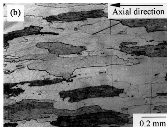
Fig. 6. Microstructures obtained after recrystallisation heat treatment at 1380°C for 1 h in tube W: (a) cross-section and (b) flat section.
