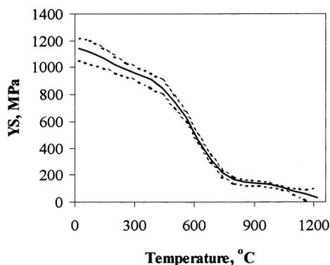
Fig. 5. Effect of the temperature on yield strength (YS) of PM2000 calculated using the method of Badmos et al. [21].
