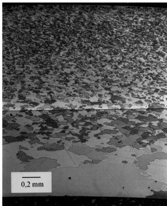
Fig. 3. Cross-section of tube R after subsequent recrystallisation at 1380°C for 1 h.
