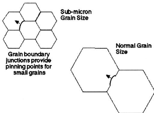
Fig. 1. The nucleation of recrystallisation occurs by the formation of a grain boundary bulge. This can occur with less constraint when the grain junctions are spaced at distances greater than the critical bulge size. With the ultra-fine grains of mechanically alloyed metals, the grain junctions are themselves pinning points, making it very difficult to form large enough bulges.
