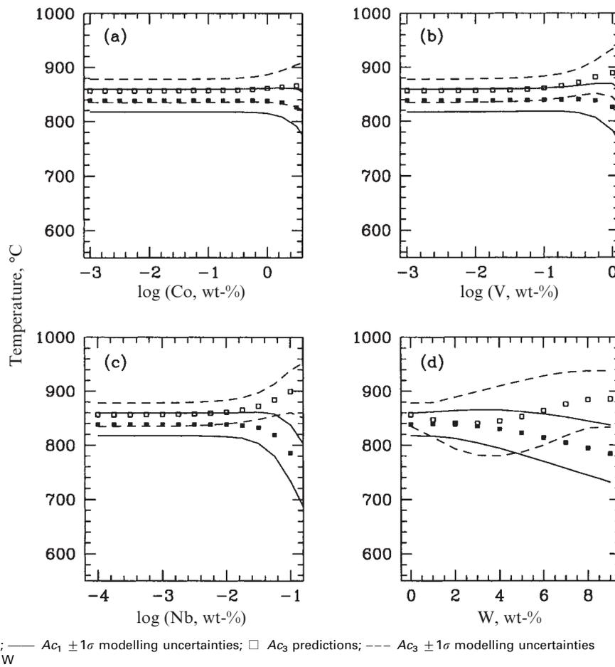
**6 Gaussian process model predictions for Co, V, Nb, and W: alloys are Fe-0.2C steels, heating rate is 1 K s<sup>-1</sup>**
