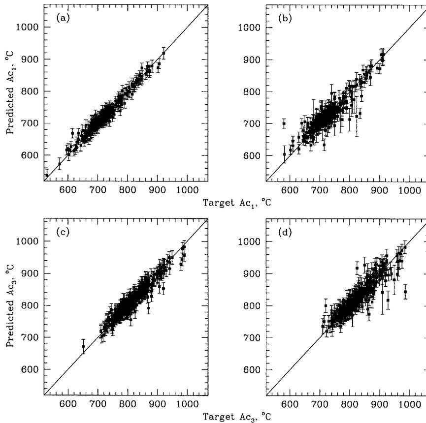
a  $Ac_1$  model predictions of training data,  $E = 11.3^\circ\text{C}$ ; b  $Ac_1$  model predictions of test data,  $E = 20.9^\circ\text{C}$ ; c  $Ac_3$  model predictions of training data,  $E = 15.4^\circ\text{C}$ ; d  $Ac_3$  model predictions of test data,  $E = 22.7^\circ\text{C}$
