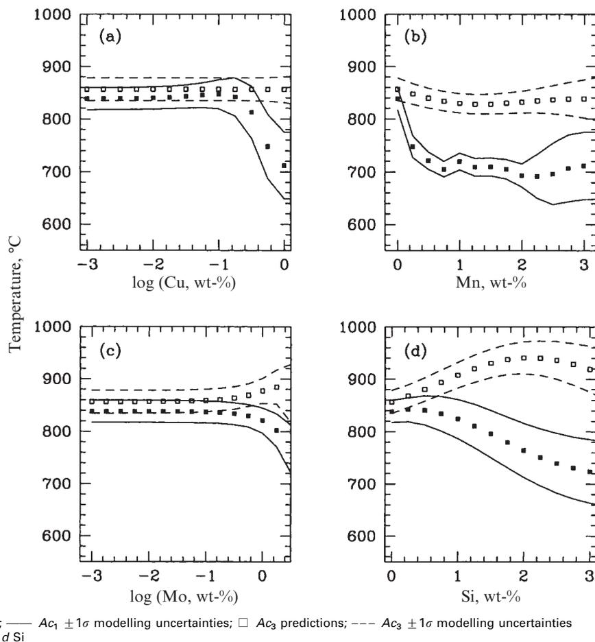
5 Gaussian process model predictions for Cu, Mn, Mo, and Si: alloys are Fe-0.2C steels, heating rate is  $1 \text{ K s}^{-1}$
