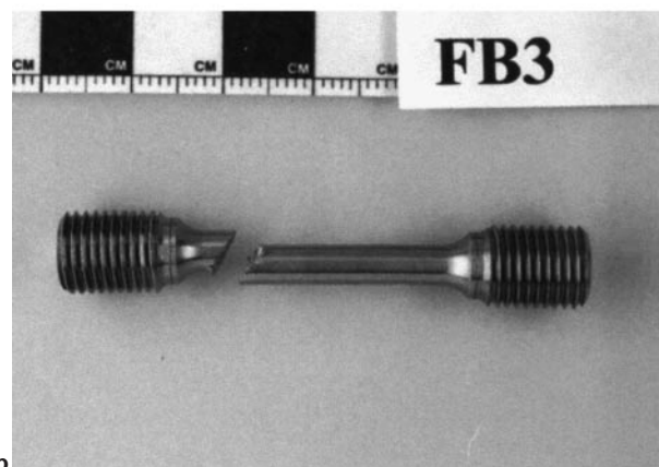
5 a tensile fracture strength results; b typical examples of failed MeMeC E and MeMeC F B specimens
