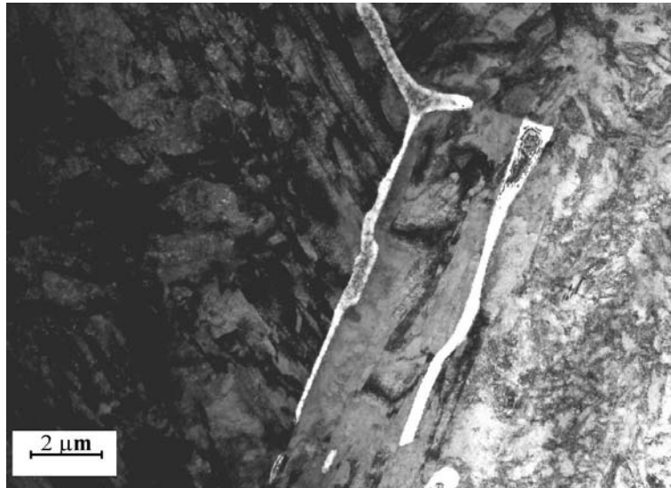
Figure 5.10: TEM micrograph showing grain boundary and intragranular \delta -ferrite found in the dual-phase HAZ of weld WAB1 side A.
