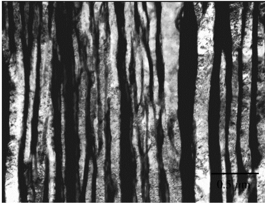
Fig. 4b: Transformed at 250° for 25 days.
