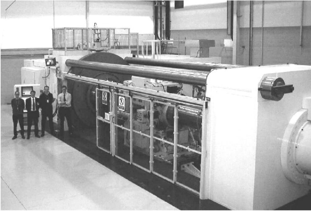
Fig. 1: 2000 ton-force inertia welding machine installed at Rolls-Royce plc near Nottingham, UK.
