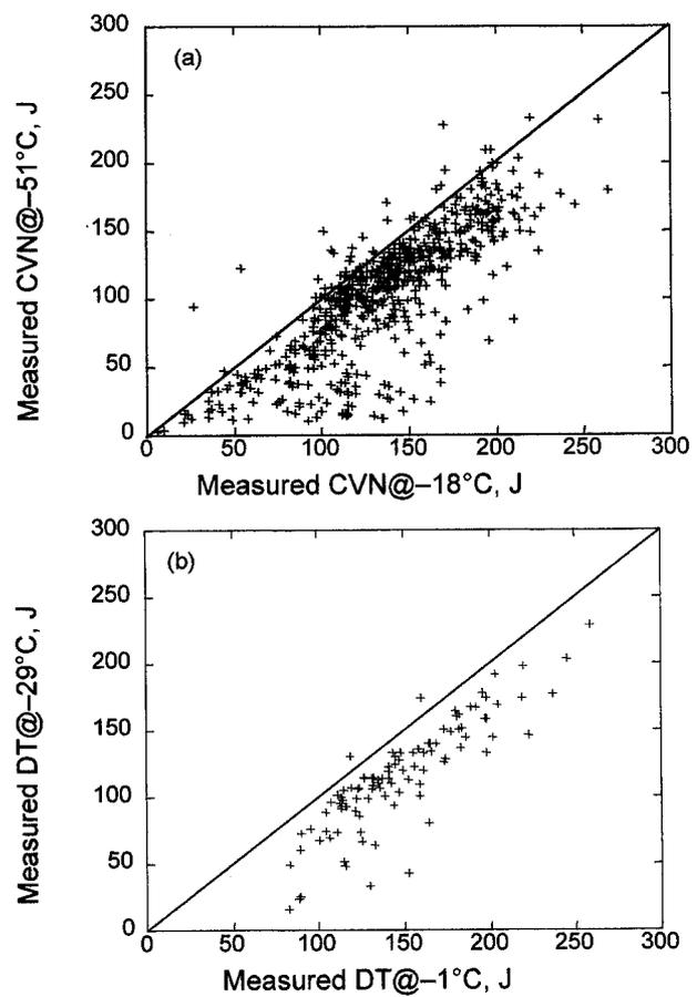
**1** Plots of *a* measured Charpy V notch energy at  $-51^\circ\text{C}$  as function of that measured at  $-18^\circ\text{C}$ , and *b* dynamic tear energy measured at  $-29^\circ\text{C}$  as function of that measured at  $-1^\circ\text{C}$
