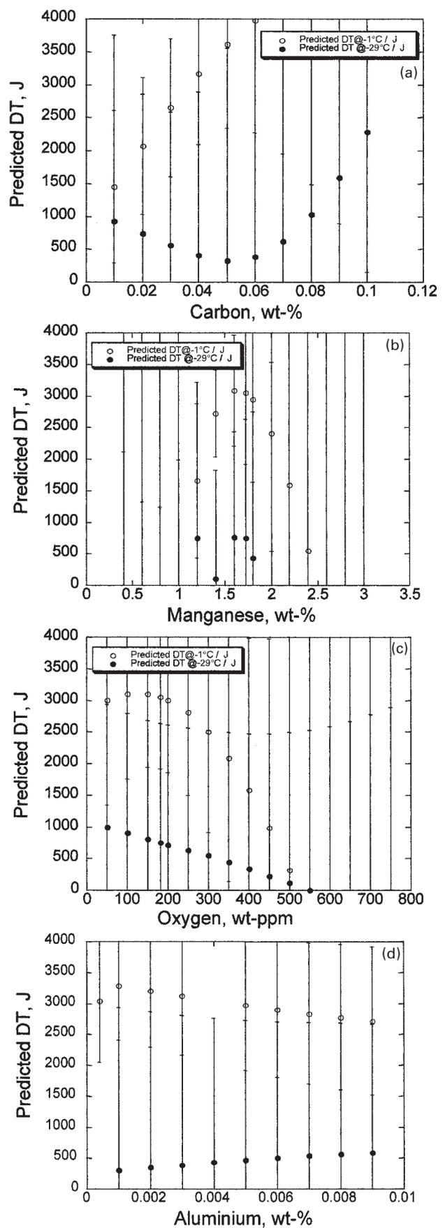
9 Variations of dynamic tear values at  $-1$  and  $-29^{\circ}C$  predicted using committee models, as functions of *a* carbon, *b* manganese, *c* oxygen, and *d* aluminium concentrations: error bars represent  $\pm 1\sigma$  values
