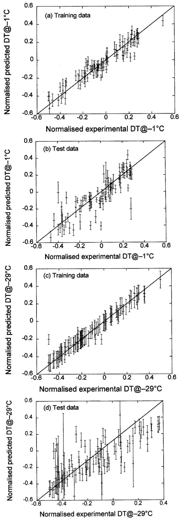
2 Predicted values using best models versus measured values for Charpy V notch tests at *a,b* -18 and *c,d* -51°C for training and test data: all data are normalised
