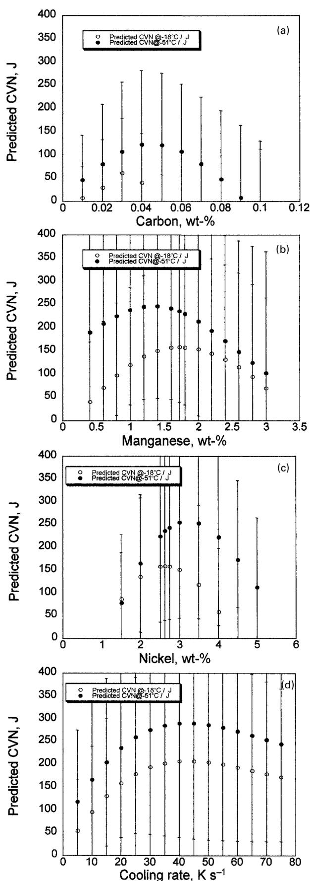
**5 Variations of Charpy V notch values at  $-18$  and  $-51$  °C, calculated using committee models, as functions of *a* carbon, *b* manganese, and *c* nickel concentrations and *d* cooling rate: error bars represent  $\pm 1\sigma$  values**
