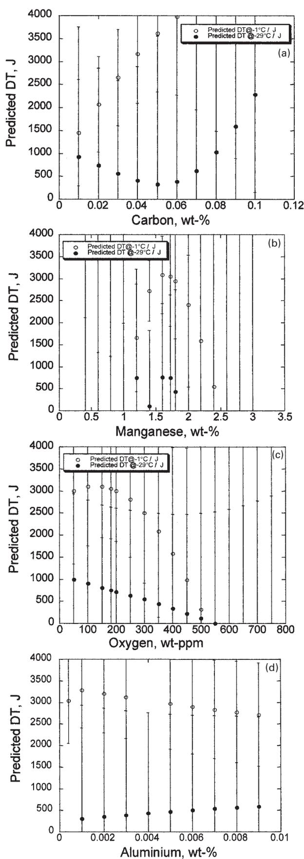
9 Variations of dynamic tear values at  $-1$  and  $-29^{\circ}C$  predicted using committee models, as functions of *a* carbon, *b* manganese, *c* oxygen, and *d* aluminium concentrations: error bars represent  $\pm 1\sigma$  values
