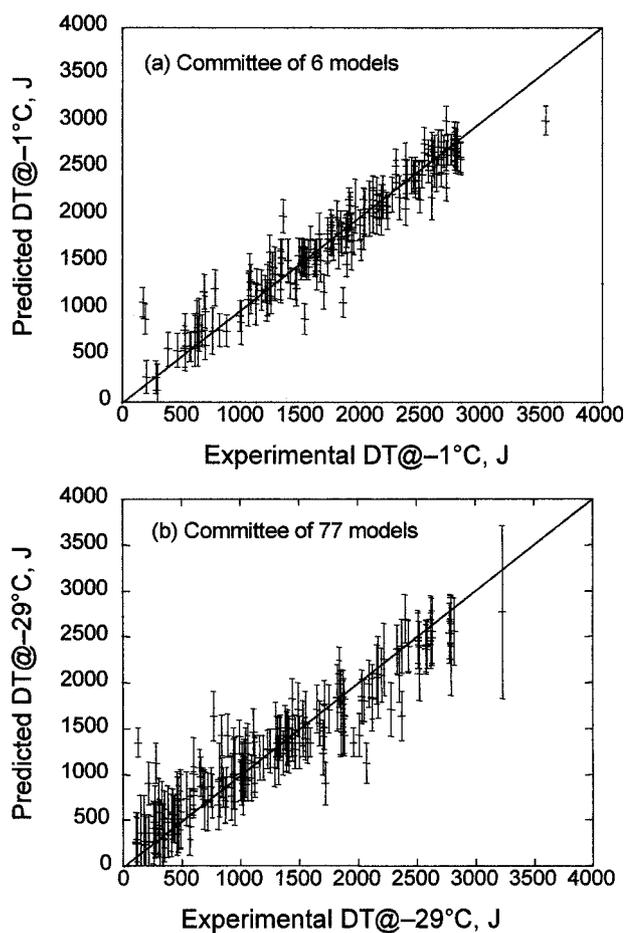
7 Comparison of predicted and measured dynamic tear values for as deposited weld metal tested at *a*  $-1$  and *b*  $-29^\circ\text{C}$ : calculations were carried out using committee models (error bars represent  $\pm 1\sigma$  values)
