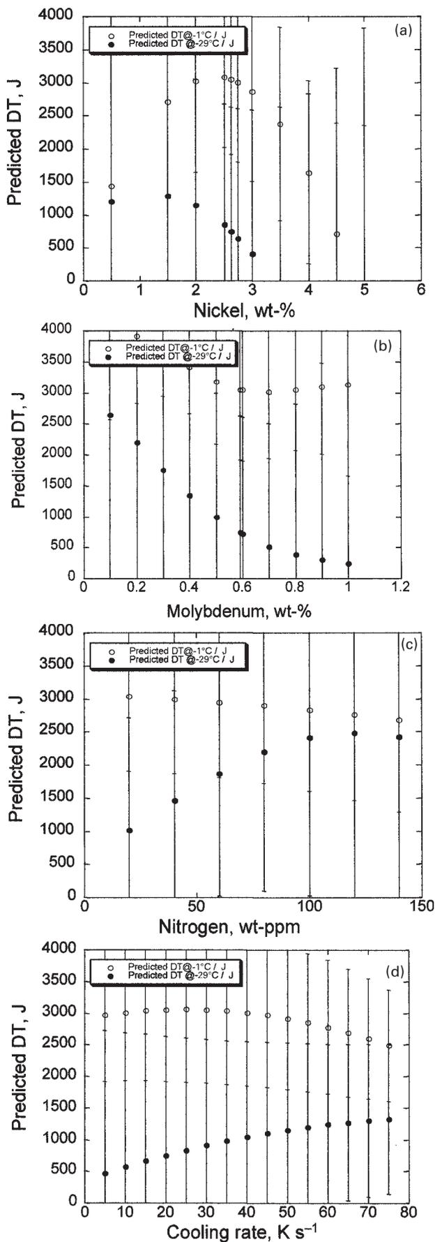
8 Variations of dynamic tear values at  $-1$  and  $-29^{\circ}C$  predicted using committee models, as functions of *a* nickel, *b* molybdenum, and *c* nitrogen concentrations and *d* cooling rate: error bars represent  $\pm 1\sigma$  values
