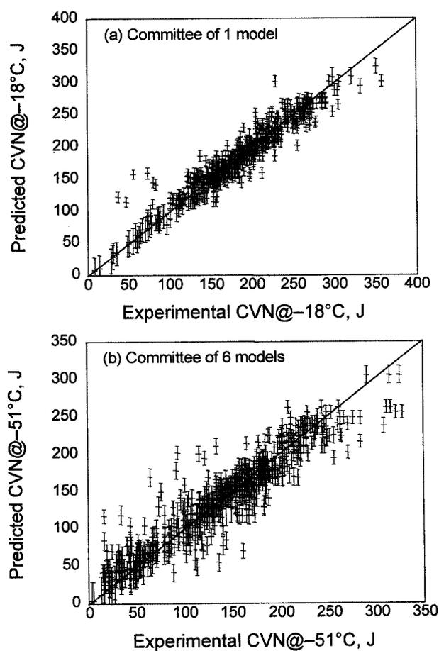
4 Comparison of predicted and measured Charpy V notch values for as deposited weld metal tested at *a*  $-18$  and *b*  $-51$  °C: calculations were carried out using committees of models (error bars represent  $\pm 1\sigma$  values, where  $\sigma$  is standard deviation)
