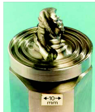
Prototype Triflute tool with three flutes and a helical ridge around the flutes' lands
