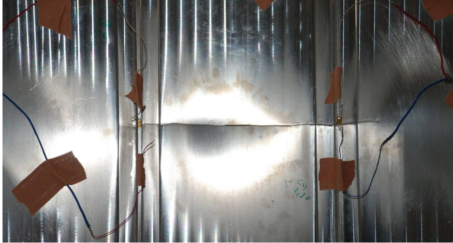
Figure 355 - Fatigue crack just outside the stiffeners.
