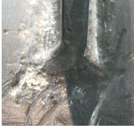
Figure 332 - Secondary crack at 17500 cycles.
