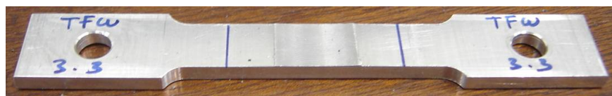
a) specimen TFW3.3 before tensile test
