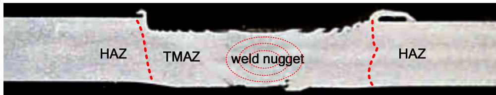
Figure 189 - Macrostructure of the FS welded AA6082-T6 containing defects.
