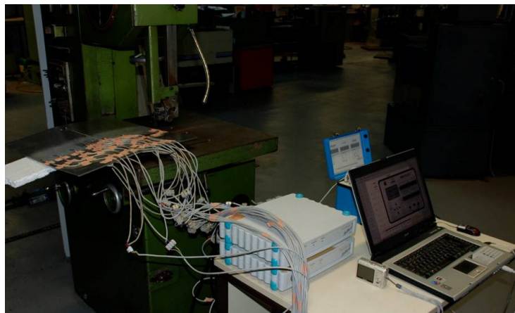
Figure 65 - Sectioning method experimental setup.
