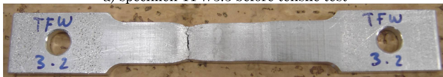
b) specimen TFW3.2 after tensile test
