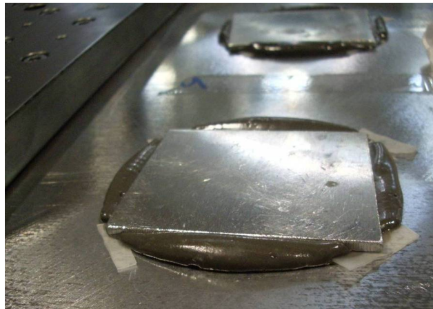
Figure 333 - Patches used to control the fatigue crack growth of secondary cracks.
