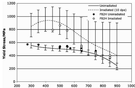
Figure 9: Model predictions for F82H compared to experimental values
