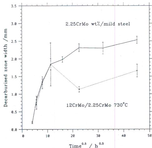
12 Decarburised zone width versus square root of time for mild steel/2.25Cr–1Mo and 12Cr–1Mo/2.25Cr–1Mo welds
