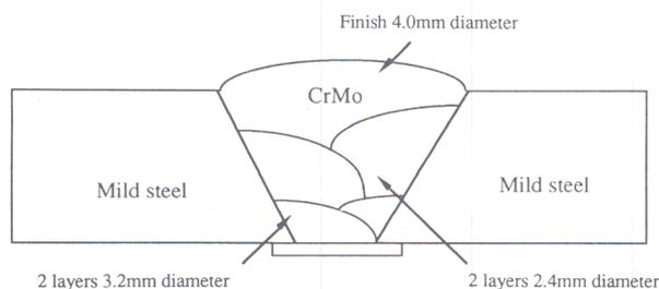
1 Welding sequence for mild steel/2.25Cr–1Mo joint
