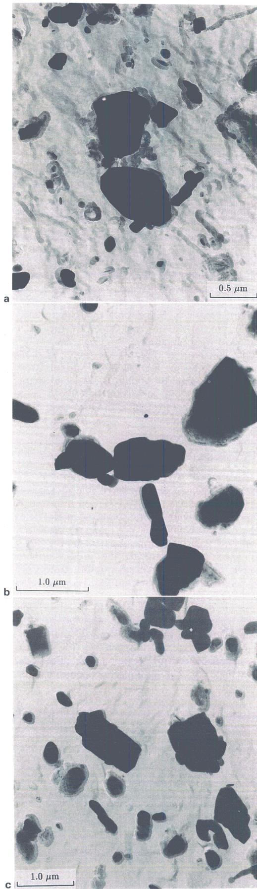
10 TEMs of 12Cr–1Mo at interface in weld held for a 16, b 256, and c 2048 h: carbide in all micrographs is  $M_{23}C_6$ , which was identified using EDX and diffraction techniques
