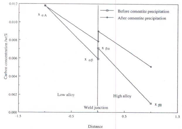
15 Calculated composition profiles for mild steel/2.25Cr–1Mo weld before and after cementite precipitation
