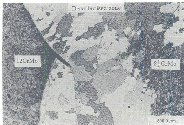
**9** Decarburised zone in 12Cr–1Mo/2.25Cr–1Mo weld held for 64 h at 730°C (optical)
