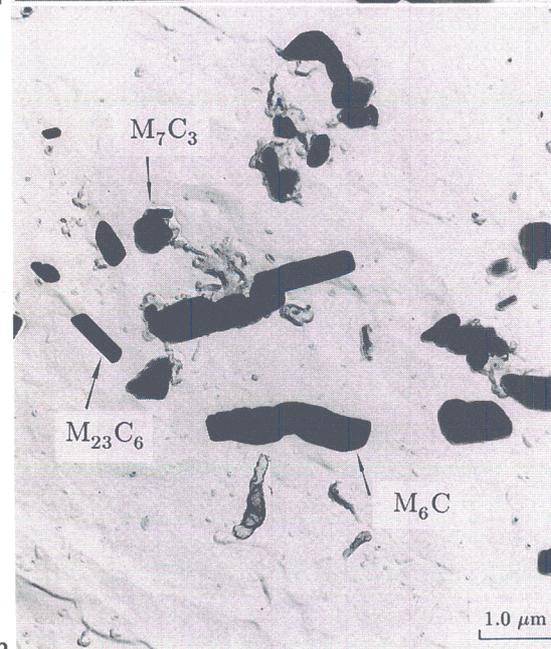
4 TEMs of region near interface in 2.25Cr-1Mo, showing morphology of carbide phases: carbides were identified using energy dispersive X-ray (EDX) analysis and diffraction patterns
