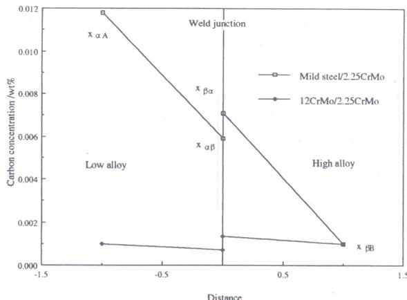
14 Calculated composition profiles for mild steel/2.25Cr–1Mo and 12Cr–1Mo/2.25Cr–1Mo welds
