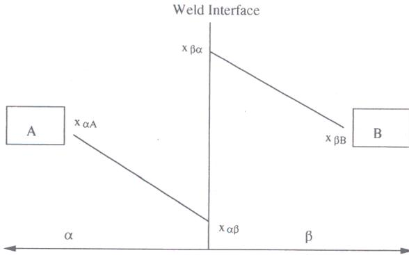
13 Schematic diagram of interfacial carbon concentrations: A and B are carbides and  $\alpha$  and  $\beta$  are corresponding ferrite matrixes having different substitutional solute concentrations
